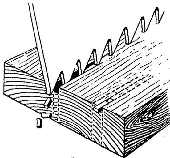
THE RIPSAW IS DESIGNED FOR CUTTING WITH THE GRAIN. THE CHISEL-LIKE TEETH CUT ON THE PUSH STROKE ONLY. SMALL PARTICLES OF WOOD ARE CUT LOOSE ACROSS THE GRAIN AND PUSHED OUT ON ALTERNATE SIDES OF THE KERF, AS SHOWN.
