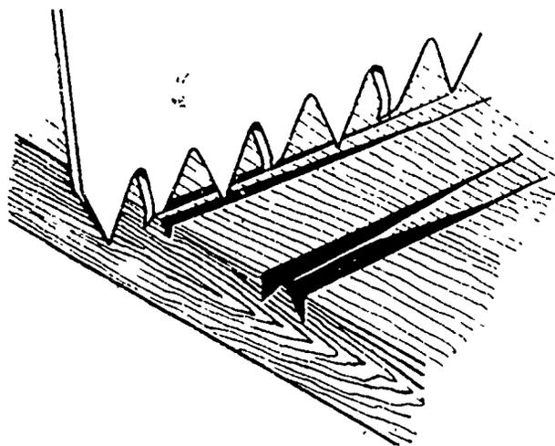
THE CROSSCUT SAW IS MADE FOR CUTTING ACROSS THE GRAIN. IT CUTS ON BOTH THE PUSH AND THE PULL STROKES. THE ALTERNATELY SET TEETH FIRST SCORE THE WOOD AS SHOWN. THEN, AS THE CUT DEEPENS, THEY PARE THE GROOVE AND CLEAR THE SAWDUST FROM THE RESULTING KERF.
