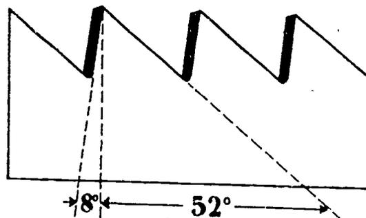
THE FRONT FACE OF A RIPSAW TOOTH HAS AN ANGLE OF  $8^\circ$ . THE BACK ANGLE IS  $52^\circ$ . THE TEETH ARE FILED STRAIGHT ACROSS THE FACE AND THUS HAVE THE APPEARANCE OF A SERIES OF CHISEL EDGES.
