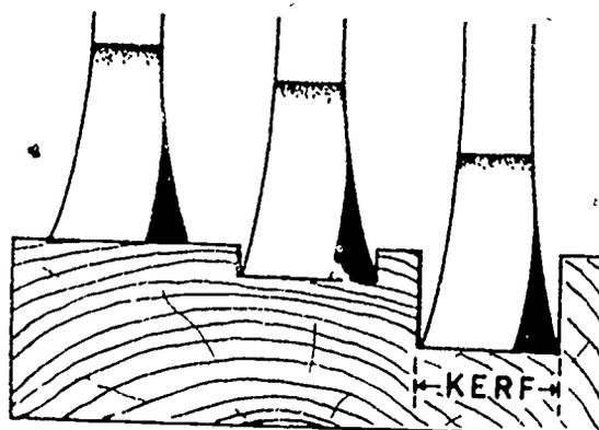
A CROSS SECTION VIEW OF THE PROGRESS OF RIPSAW TEETH THROUGH WOOD SHOWS THE CHISEL-LIKE ACTION OF THE TEETH.
