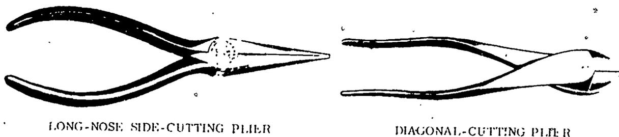
Fig. E-38. Cutting pliers
