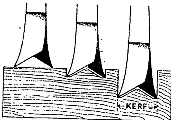
A CROSS SECTION VIEW OF THE PROGRESS OF CROSSCUT SAW TEETH THROUGH WOOD SHOWS THE KNIFE-LIKE SCORING ACTION, THE PARING ACTION, AND THE FULL CUT.
