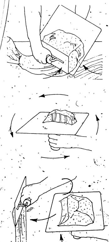
up with the mortar on top of it (you are putting the mortar onto the trowel with the hawk.
