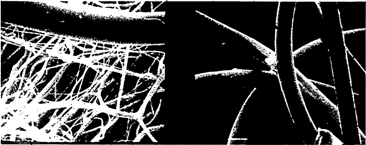
This comparison of 3M's Thinsulate® (left) and polyester (right) shows how Thinsulate's micro-fibers can trap more air in a given space, resulting in a more efficient insulator.
