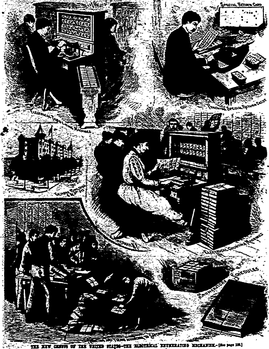
THE NEW Census OF THE UNITED STATES—THE ELECTRICAL REGISTERING MACHINERY.—(See page 128.)
