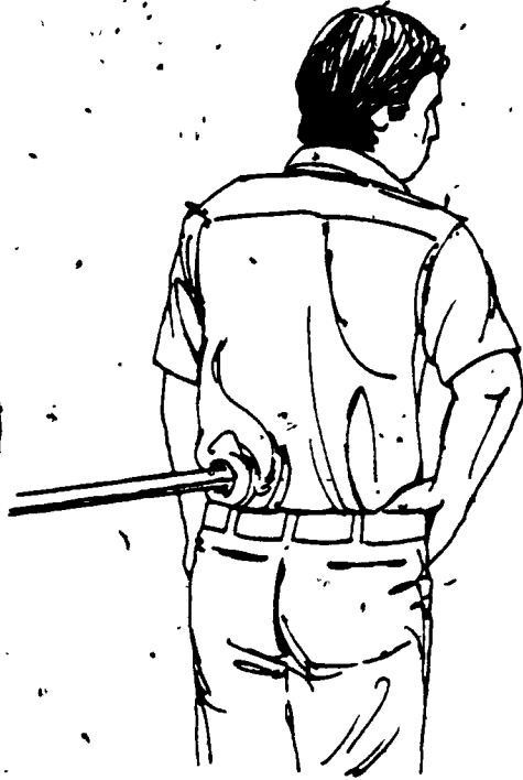
Figure 3. Contact with protruding machine parts can cause dangerous wrapping.
