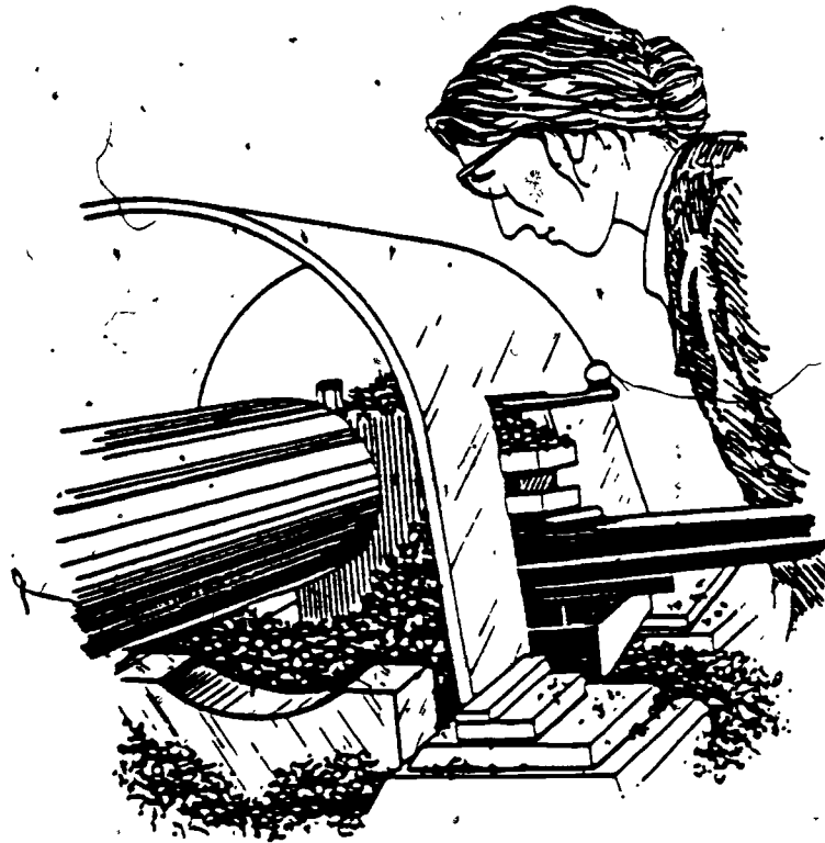
Figure 9. Lathe guard protects worker from flying chips.
