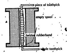
· The racer's "engine" is a twisted rubberband
