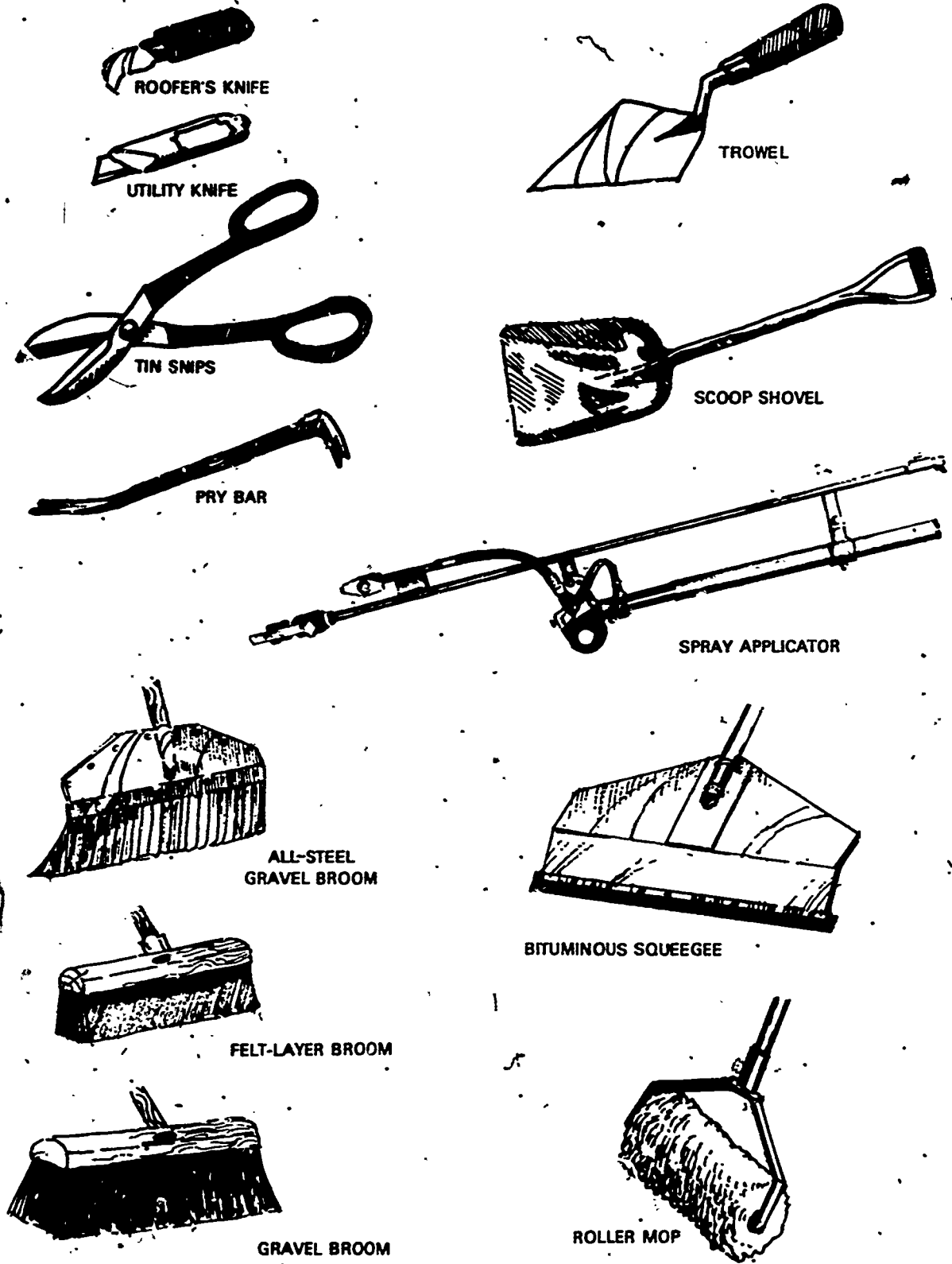
Fig. 2-1. Some tools used in cold-applied roofing and waterproofing
