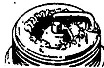
Dry, black fluffy deposits indicate gas fouling. Adjust carburetor idle mixture. If you still have gas fouling, change carburetors. (Be sure drivers are not overchoking.)
