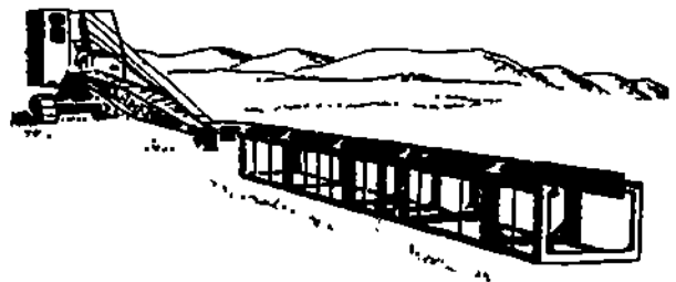
143.18 Figure 16-55.—Leads on ground and attached to boom with adapter.
