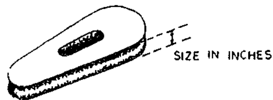
Figure 5-14.—How to measure a wedge.
