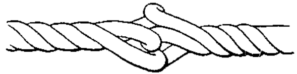
Figure 5-4.—Result of a strong strain on a line with a kink in it.
