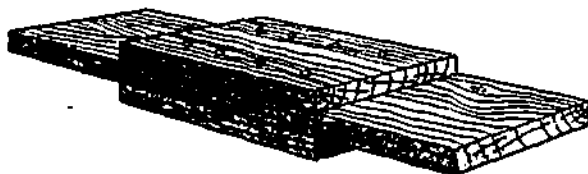
68.38.1 Figure 4-15.—End butt joint with fish plates.
