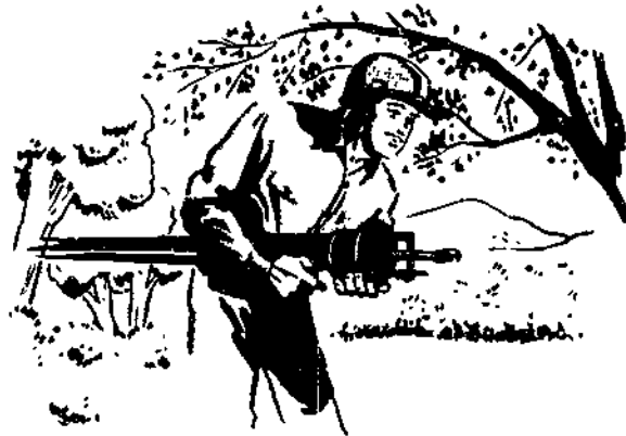
Figure 6-10.—Safest carrying position for instrument when obstacles may be encountered.
