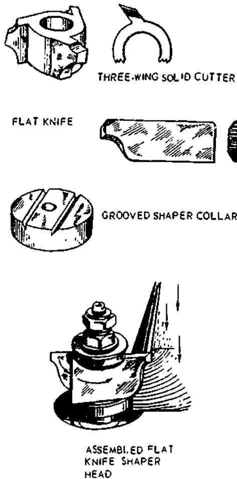
Figure 3-54.—Three-wing cutter and flat knives for a shaper.
