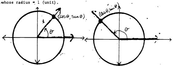
Any point, A, on the unit circle has coordinates  $(\cos \Theta, \sin \Theta)$  where  $\Theta$  is the measure of the angle whose terminal side passes through A.
