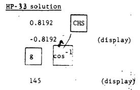
Thus  $x = 145^{\circ}$  is <u>one</u> root of this equation. In general, the <u>principal</u> value of an inverse trigonometric function is:
