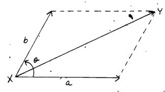
include an angle whose measure is . In our diagram the magnitude of the resulting force is the length of diagonal XY. The forces a and b are known as components and force XY is called their resultant. The process of finding the resultant of two or more forces is called determining the parallelogram of forces. The forces themselves are called vectors because they have a specific magnitude and direction.
