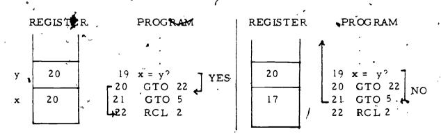
The TI-57 does not have a y-register so a special store called a t-register is established. A number is placed in the t-register, R<sub>t</sub>, by use of the x x x t key. Thus if we wish to place 20 in R<sub>t</sub>, we merely
