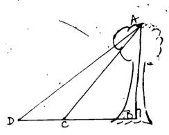
ADB is the angle of elevation of the top of the cliff from D.
