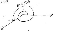
The values of the trigonometric function for 563° are the same as for 203° because the initial and terminal sides of both of these angles coincide.
