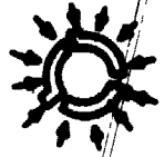
wafer (example shown: 3-pole, 3 circuit with 2 nonshorting and 1 shorting moving contacts)
