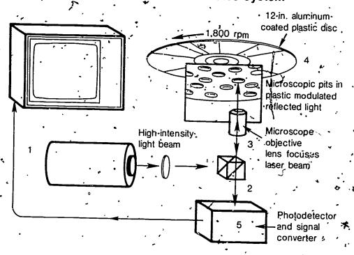
Figure 3. Optical effective videodisc system diagram. Numbers one through five show the path of the laser beam from the high-intensity light beam to the surface of the optical reflective videodisc and the reflected beam through the lens to the signal converter for display and sound on a television receiver or monitor.
