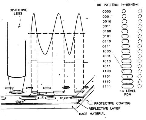
Figure 4. Data storage on videodisc. The bit patterns for storing digital data on optical videodisc are graphically represented here. Digital data storage on the optical videodisc makes it one of the most dense storage mediums at this time.
