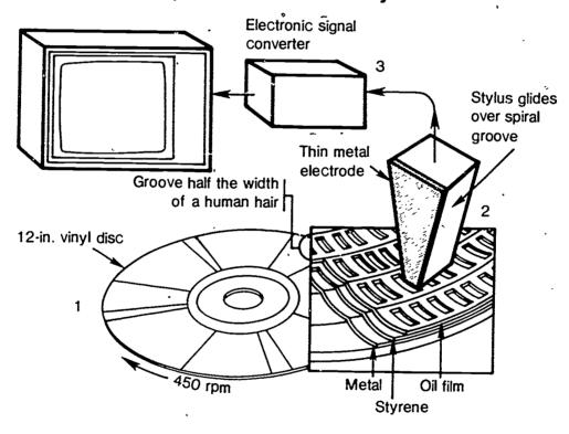
Figure 6. Capacitance videodisc systems diagram. The capacitance (mechanical stylus) system was earlier introduced on the TED videodisc systems, and most recently used with the RCA Selectivision Videodisc System to be introduced in 1981 to the general home video markets. It will produce an adequate video signal, but is limited in "search and freeze frame" because of the apparent wear on the disc when played other than linearly.
