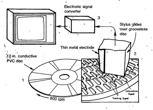
Figure 7. Combined optical/capacitance system diagram. The combined system has been used primarily by the Victor Company of Japan (JVC), and provides for a grooveless disc which is tracked by a laser and the signal taken from the disc by a mechanical stylus which "floats," making slight contact with the disc. This system has yet to be marketed in the United States but appears to be nearing release.
