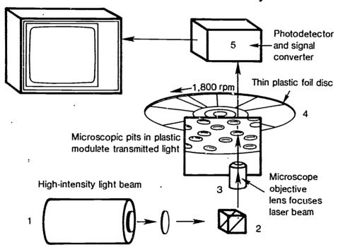
Figure 5. Optical transmissive system diagram. The high-intensity light beam in this system is not reflected, but rather passes through the transparent videodisc carrying the signal to the converter and to the television receiver or monitor. This system is very stable under conditions of movement or stress while it is in operation, e.g., in a military tank or other rough riding vehicle.
