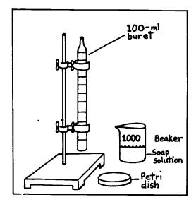
While the pump is warming up, prepare the bubble meter for use.
