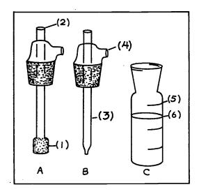
The bubbler is identified by its frit--a porous piece of glass at the end of the inlet tube.
