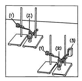
Calibrate the sampling train just prior to sampling with it. Set up another impinger and filter as a blank.
