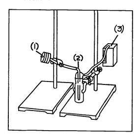
The sampling train consists of three major components: a filter, a trap, and a pump.
