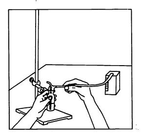
Do not spill the absorbing reagent while attaching the tubing.
