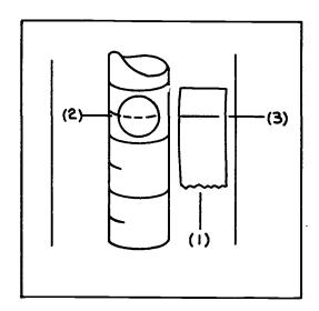
Make a mark on the tape to show where the center of the rota-meter ball should be when the pump is drawing the desired flow rate.
