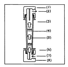
Use a precision rotameter if the pump you use does not have a flow meter built in.
