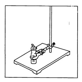
Add distilled water to the impinger bottle, grease the ground-glass surfaces, and clamp the impinger.
