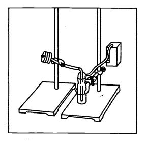
Hold the filter assembly with a ringstand and shaft clamp. Do not tighten the clamp on the tubing; just rest the tubing in the clamp.
