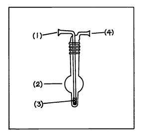
The smog bubbler has a large mixing chamber to ensure complete mixing between smog particulates and the absorbing reagent.
