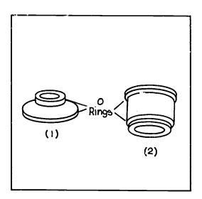
The packing usually consists of rubber 0-rings.
