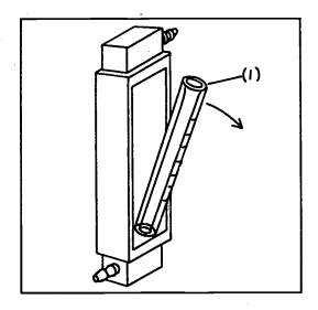
Tilt the tube forward to remove it; remove the stops and float.
