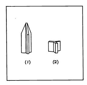
The float stops keep the float from hitting the bottom and top of the tube.
