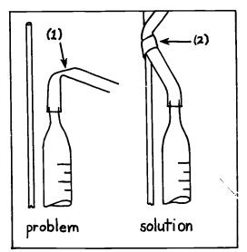
Remove the kink by supporting the tubing on the buret stand shaft.
