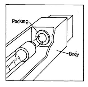
Check the O-rings and replace if necessary.
