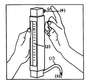
Feel the pressure of air escaping through the outlet. To push the float up to the top of the scale, the air pressure must be 10 times greater than when it is at the bottom.
