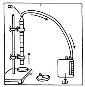
Connect the tubing so that air flows into the sampling device through the tubing and into the pump.
