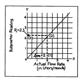
Plot each "1" against each corresponding "R" to find the relationship between an actual flow rate value and the corresponding rotameter reading.
