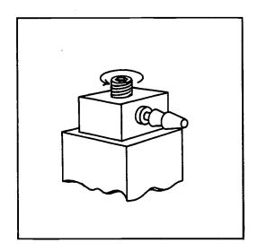
Do not remove the jack screw completely.
