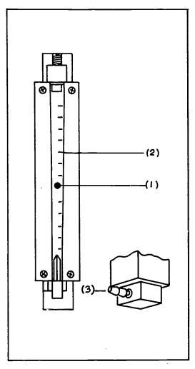
The float travels through a tapered tube.
