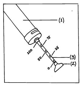
Marks on the shaft indicate air volumes that can be drawn into the pump.
