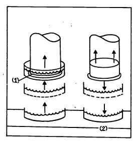
After pulling the handle out, lift the dish to form a bubble; lower it quickly when one has formed.
