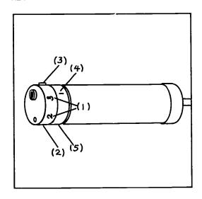
Index numbers on the edge of the rotation head correspond to orifices in the flow control plate.
