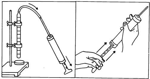
You will learn to calibrate and use a detector tube sampling pump in three lessons:
