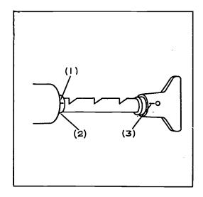
A volume of 50 ml is drawn into the pump when the rotating head is set at "3" and the handle pulled out to "50 cc."
