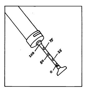
Pull the pump handle out to the mark equal to the volume pulled at each orifice Setting.
