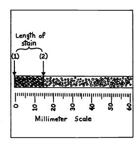
Measure the length of stain using the color-millimeter scale.
