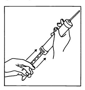
When an unopened tube is inserted in the pump, guide the pump handle back to its starting position to prevent damage to the pump.
