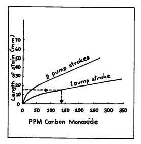
To determine CO, first select the pump stroke curve. Read the length of stain on the vertical line, move straight to the curve, and straight down to the horizontal line. Read ppm CO.
