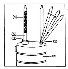
Break off the tips of the detector in the breaker hole. Discard the glass pieces in a waste container.
