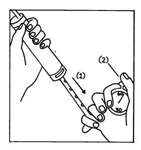
By checking the flow rate of the pump, you can test whether the orifices are clear.
