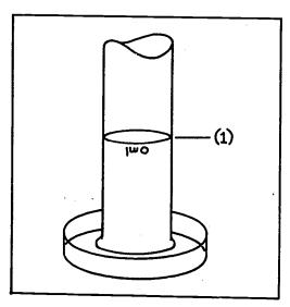
Before beginning to calibrate, line up a bubble on the 0-ml mark.
