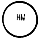
Hot Water Heater
