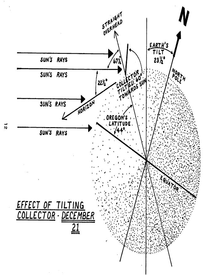
7. The sun is at about a  $60^{\circ}$  angle south of straight overhead at noon in the winter in Oregon, so a solar collector used for winter heat should be tilted up off the ground at about a  $60^{\circ}$  angle toward the south.
