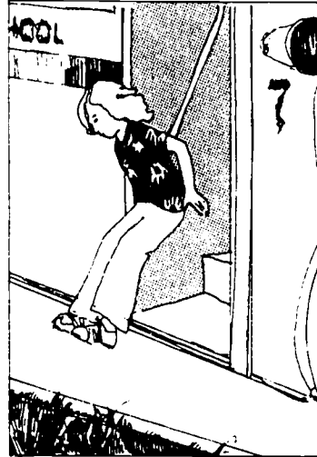
Fig. 2. Removing children safely from bus that has live electrical wire on it
