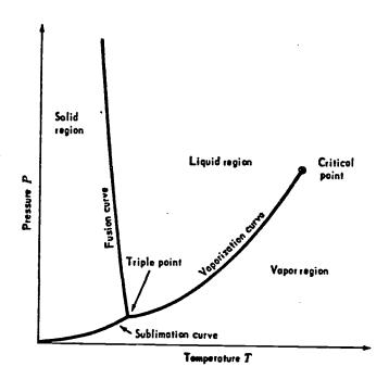
Figure 1. A pressure-temperature diagram for a substance such as water. The triple point is the point of intersection of the sublimation, fusion and vaporization curves. From Zemansky, M.W. and H.C. Van Ness. 1966. P. 200.
