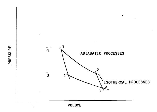
Figure 4. Pressure-volume diagram. A cycle is composed of going from 1 to 2, 2 to 3 and so on back to 1. When the cycle is composed of isothermal and adiabatic processes it is called a Carnot Cycle. Other cycles can involve constant pressure or constant volume steps. Note that T<sub>1</sub> is greater than T<sub>2</sub>.
