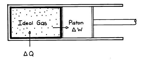
Figure 3. Ideal gas contained in a piston chamber.  $\Delta Q$  will be zero if the wall surrounding the system is perfectly insulated (adiabatic).  $\Delta W$  represents the change in work accomplished by moving the piston.
