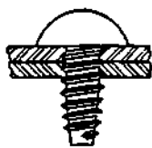
IN DRILLED OR CLEAN PUNCHED HOLES
