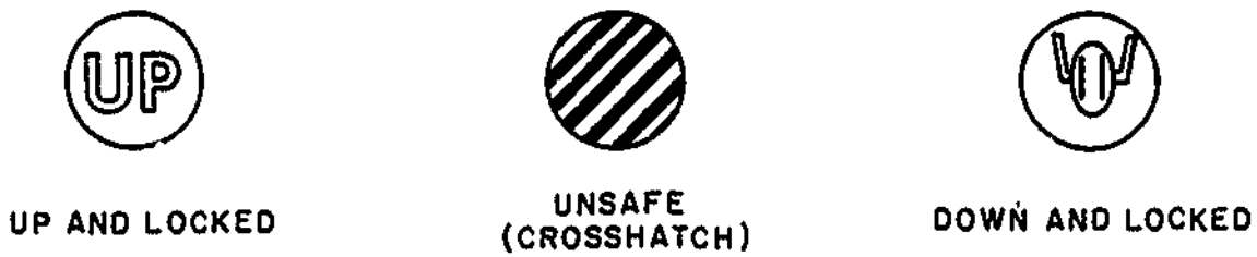
Figure 2. Wheel Position Indications.
