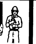
TRAVEL Right hand in front of body, making a walking motion about face while indicating direction of travel, forward or backward (for greater crane body).
