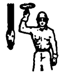
HOIST Right forearm extended, hand open, palm facing forward, fingers spread, thumb pointing upward.
