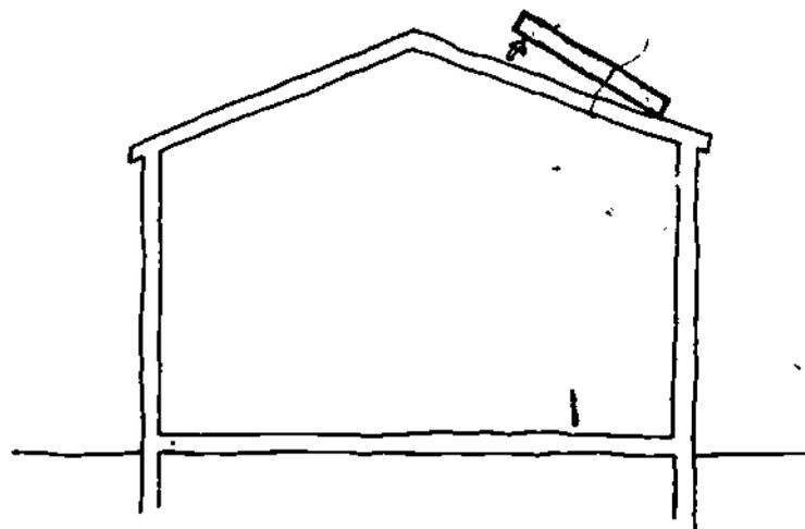
8. A collector array placed over the ridge line will usually make the installation dominate the roof.
