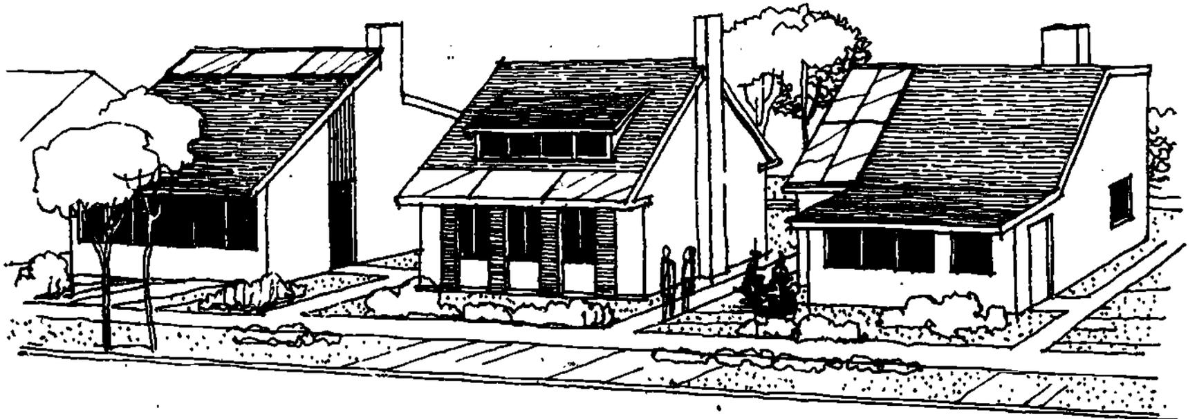
Figure 35 A Collector Array Covering an Entire Roof
