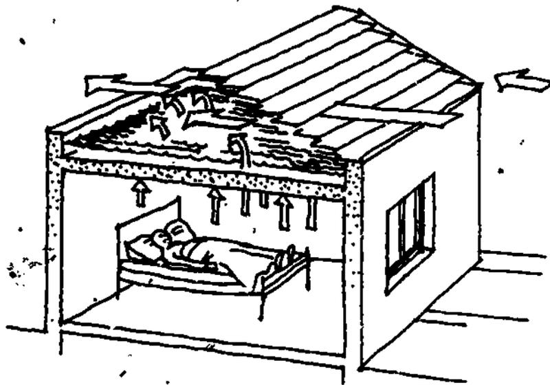
Figure 17 Solar Chimney
