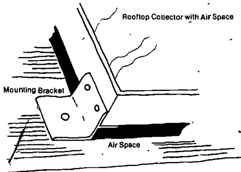
It has become widespread practice to mount roof collectors an inch or so above the roof as illustrated. This will allow rainwater or melting snow to pass under the collectors, and avoids the difficulty associated with caulking and the visual objections with metal flashing, normally associated with inlaid and flat-on-the-roof type mountings.
