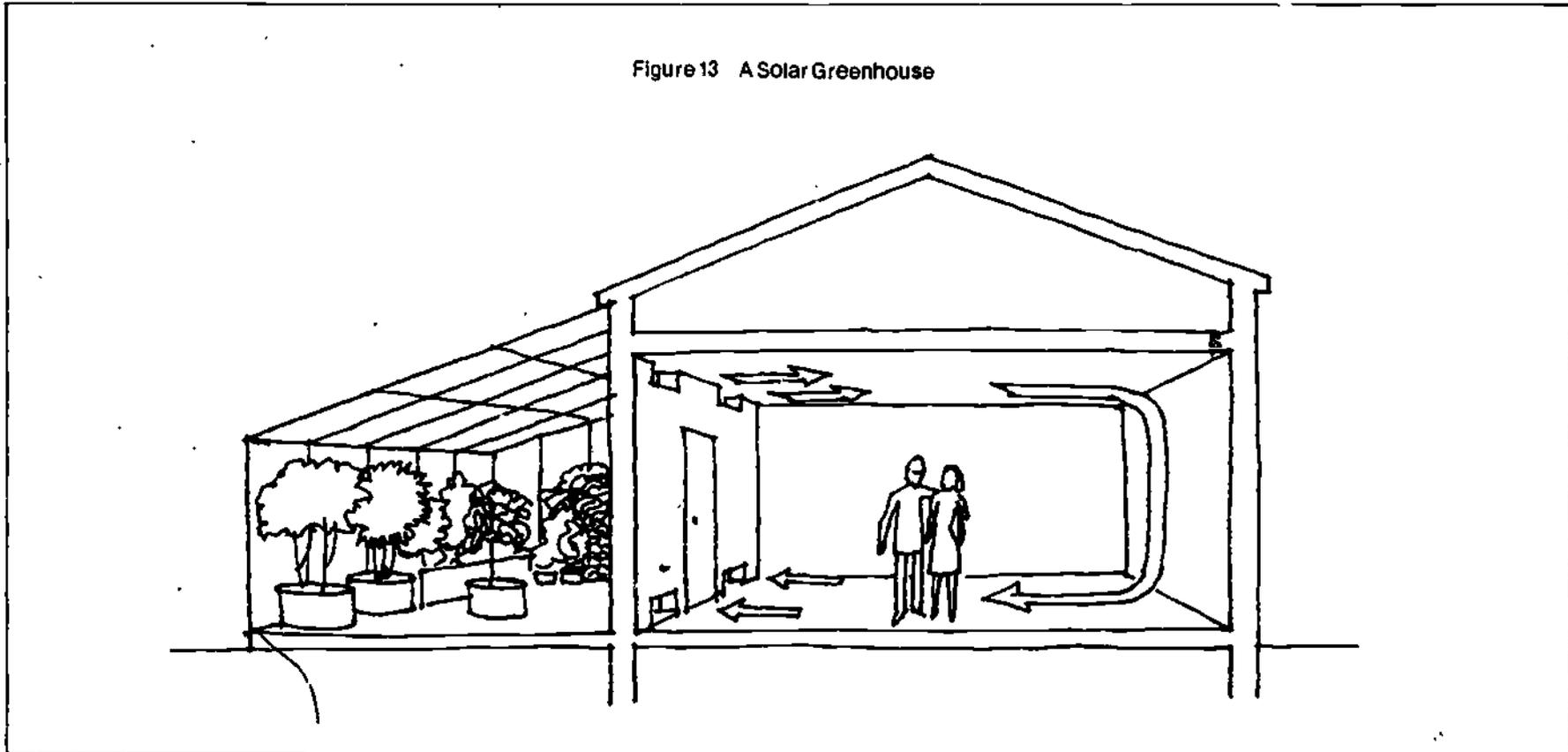
A greenhouse is an especially useful means of retrofitting an existing building with a passive solar system. Greenhouses are aesthetically acceptable to most people and, when properly located and built of compatible materials, they can add significantly to the appearance of most buildings.
