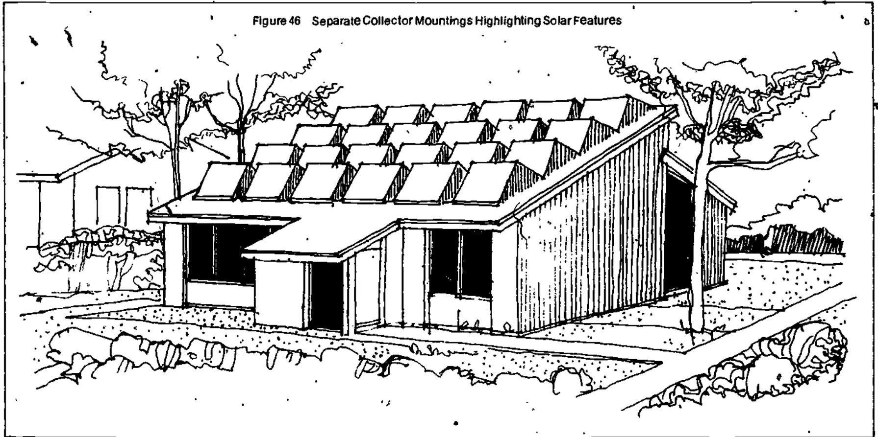
Figure 46 shows a variation of this idea. In this actual retrofit installation, the individual collectors are not installed as one continuous array. Instead, each collector module has its own separate mounting. This installation creates a unique and dramatic design that highlights the solar system. Modifications of this approach, less radical in appearance, are possible for a wide range of housing styles, provided that the building is compatible with neighboring homes and buildings.
