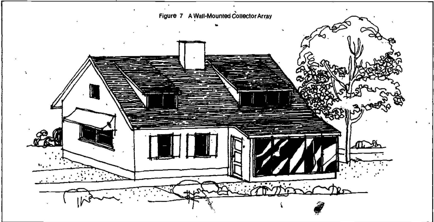
tem where a building's roof is not pointing south, but the roof of the garage is.
