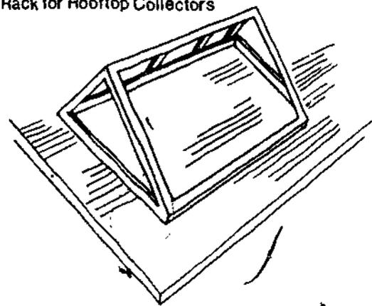
Rack-Mounted Rooftop Collectors with Enclosures
