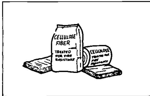
FIGURE 24. Cellulose fiber is supposed to be treated by the manufacturer for fire and vermin resistance.
