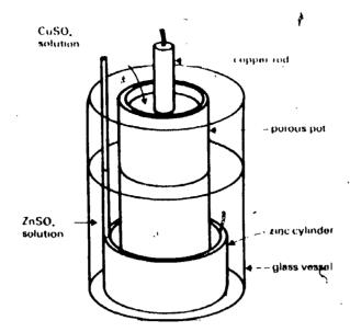
$E^{0}$  cu<sup>1</sup> cu = 0.34 V<sub>a</sub>  $E^{0}$  sol so<sub>1</sub> = 0.20 V  $E^{0}$  zn<sup>1</sup> · zn = 0.76 V
