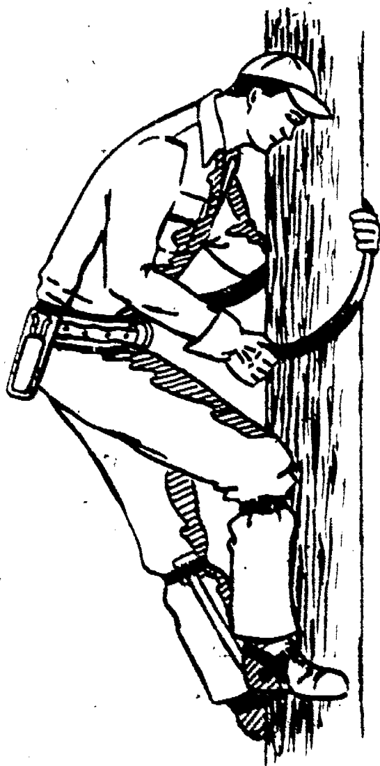
Figure 36. Transferring safety strap.
