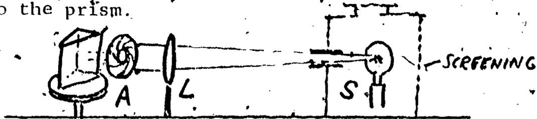
The quality of the beam transmitted through this aperture can be observed on a distant screen, L meters away, where it should appear as a uniform disc of light of diameter L cm; and this diameter should be more-or-less independent of the size of the opening A.
