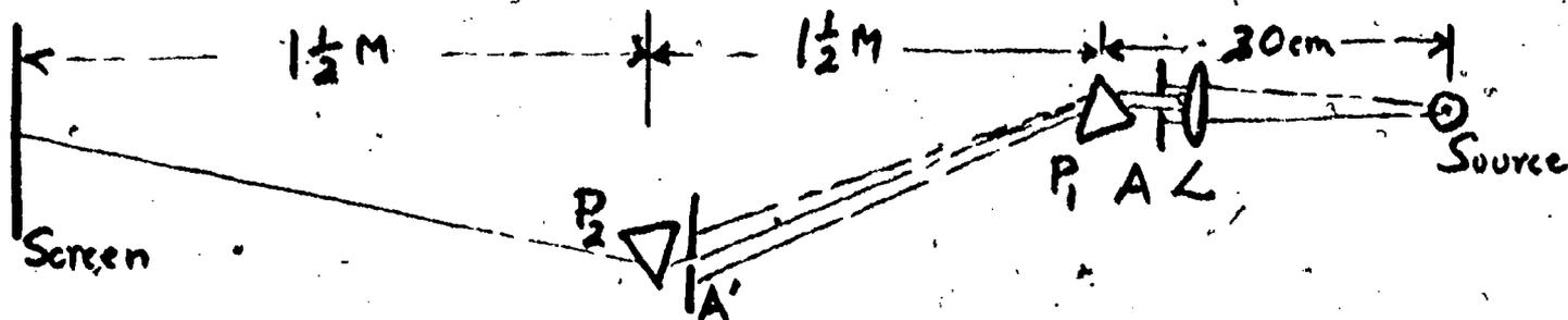
With the layout approximately as shown, the length of the spectrum at the second aperture, 'A' will be about 6 cm. and width about 2 cm. (Aperture A about 6 mm. less). A' should be an adjustable slit, with
