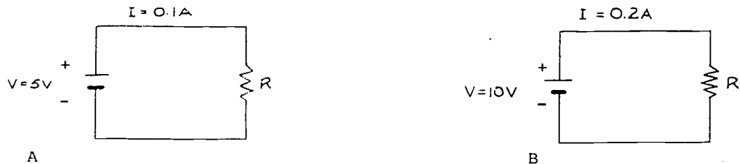
FIGURE 2: An increase in voltage causes a proportionate increase in the current in a circuit, as long as the resistance remains constant.
