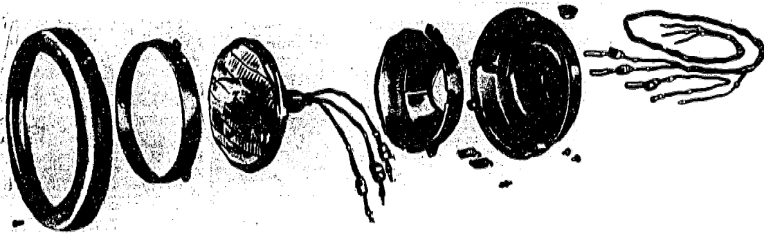
Figure 7-28.—A typical sealed beam headlamp assembly.
