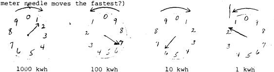
The preceeding meter reads 1662 kwh.
