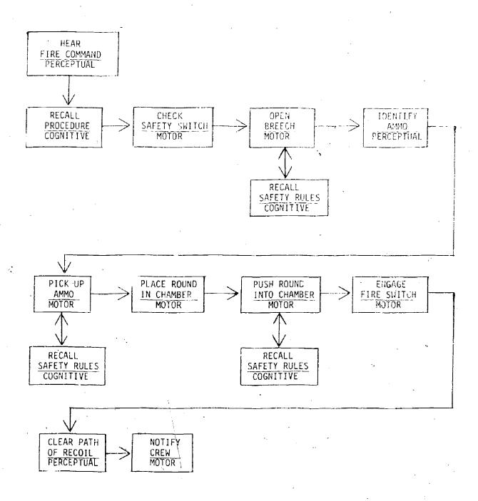
Figure 3. Response components for task: Loading round into main gun on an M60Al tank.
