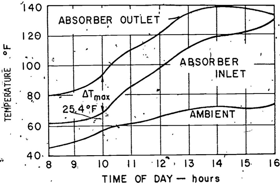
Figure 7-8. Absorber and Tank Temperatures for Thermosiphon Flow During a Typical Day
