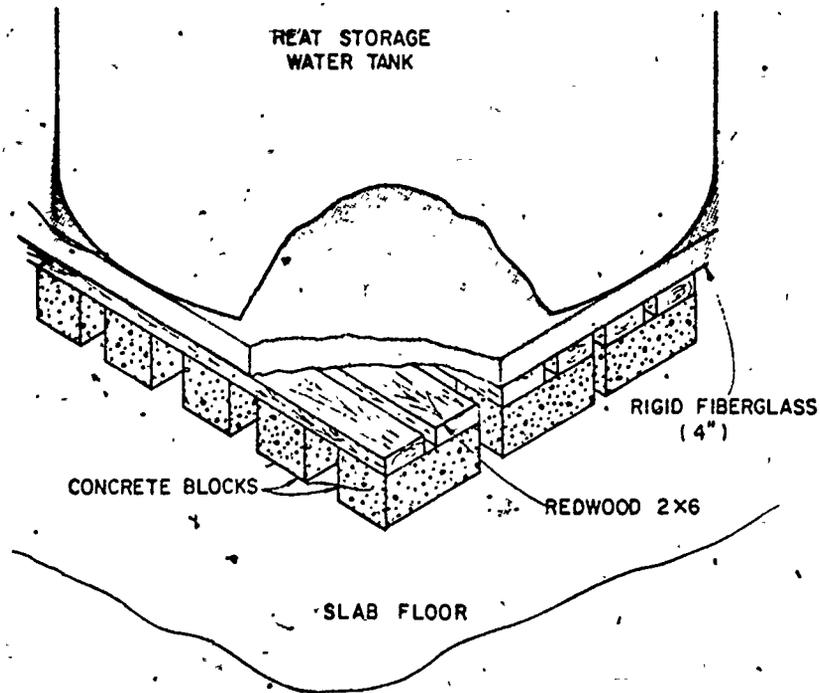
Figure 6-2. Bottom Insulation and Support Scheme for Water Storage Tanks
