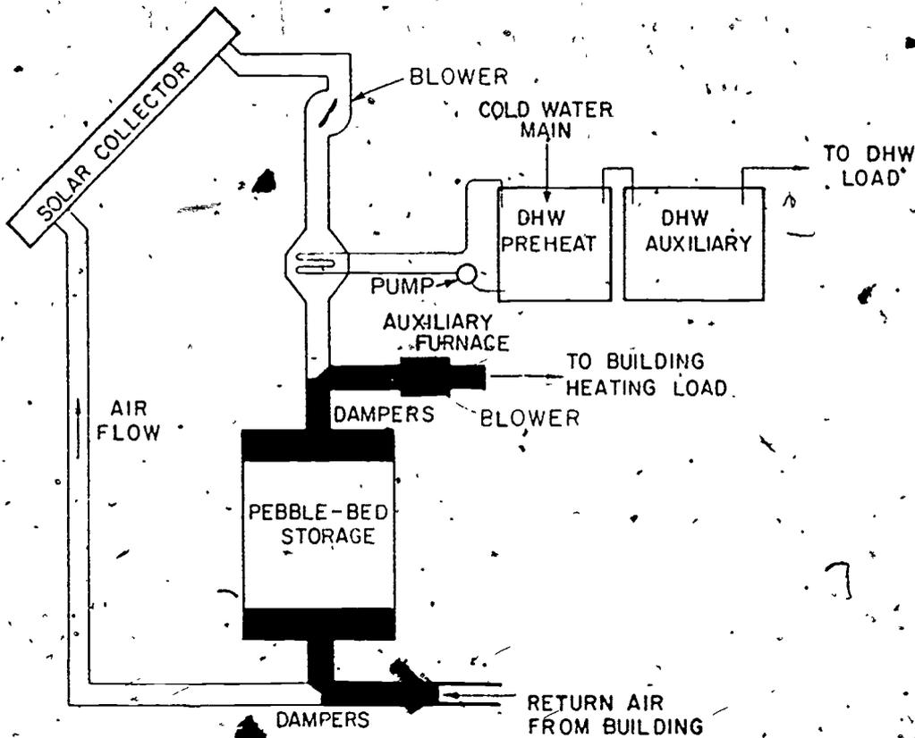
Figure 3-10. Heating from Storage
