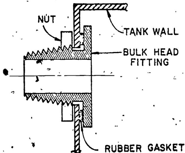
Figure 6-3. Bulk Head Type Connection
