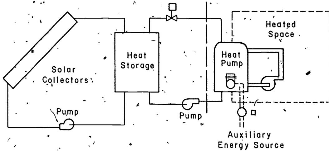
Figure 8-14. Simplified Diagram of a Solar Assisted Heat Pump System Series Arrangement
