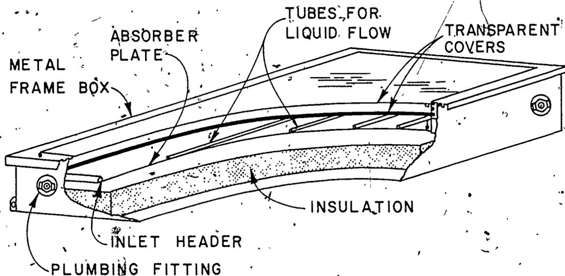
Figure 5-2. Solar Collector Module
