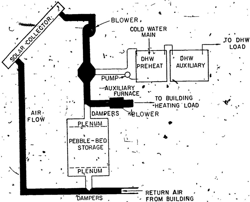
Figure 3-8. Heating from Collector
