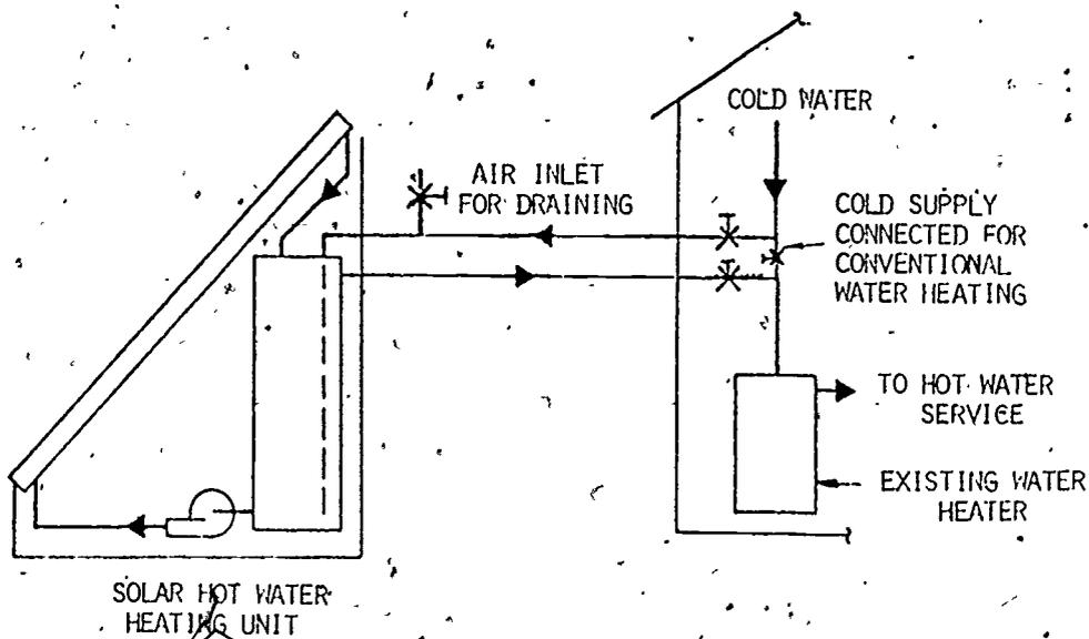
Figure 18-1. Retrofit Solar Domestic Hot Water Heater, Non-Freezing Climates
