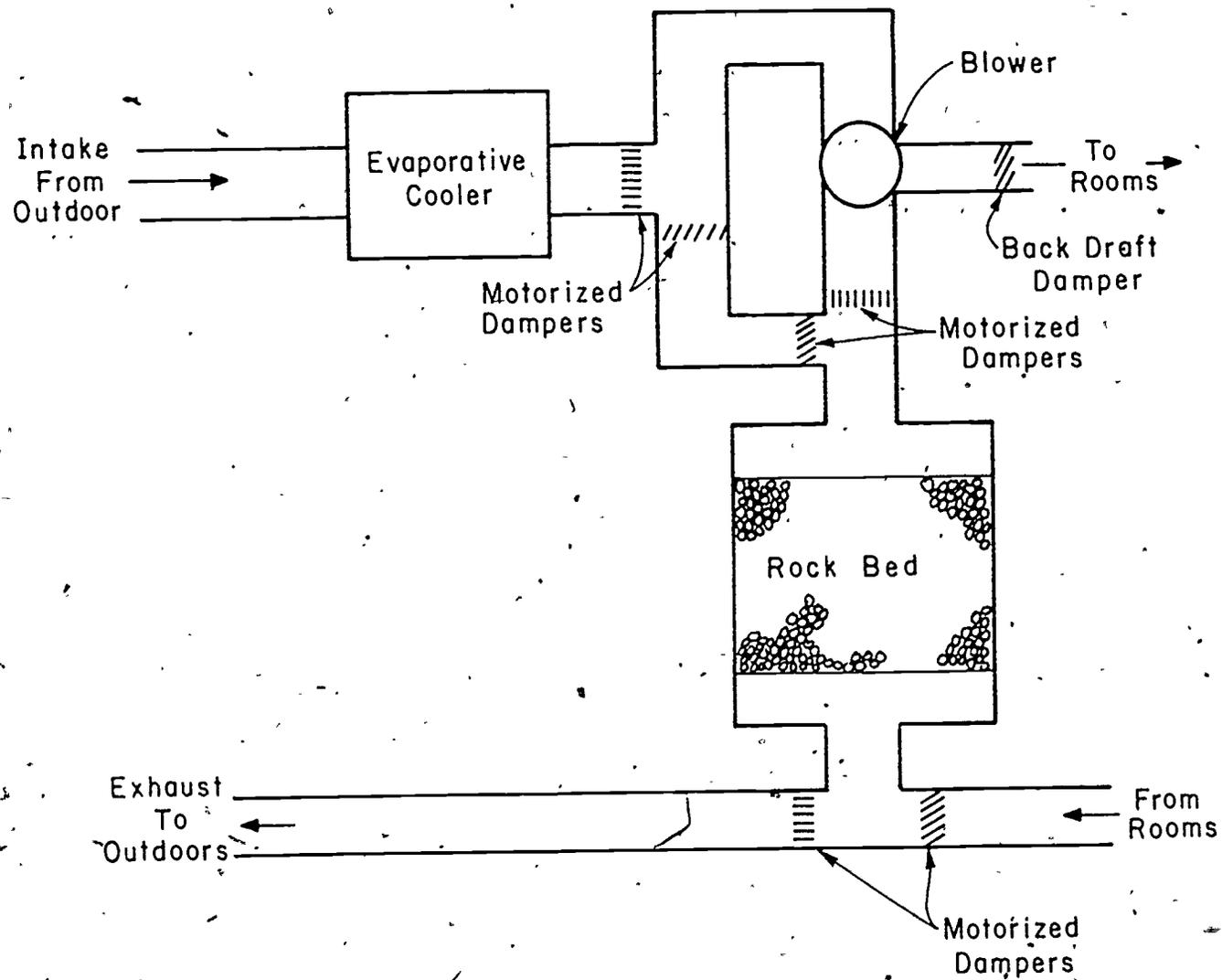
Figure 9-3. Evaporative Cooling with Rock Bed Storage
