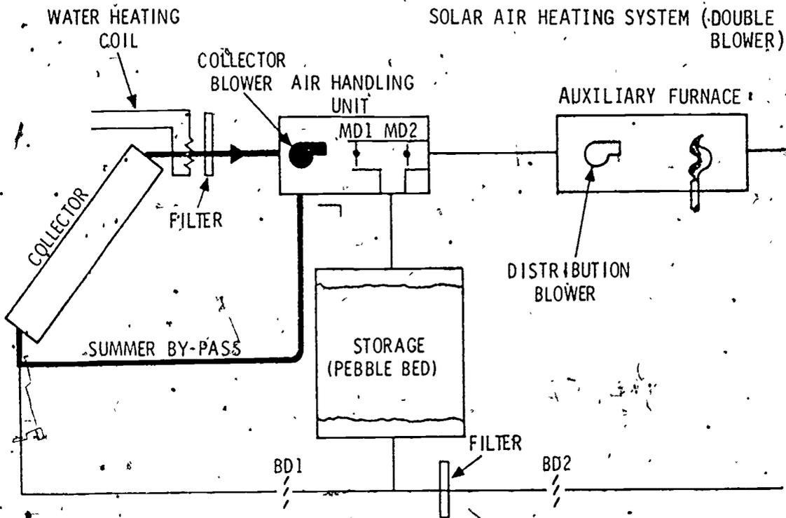
Figure 8-8. Service Hot Water Heating (Summer Operation)
