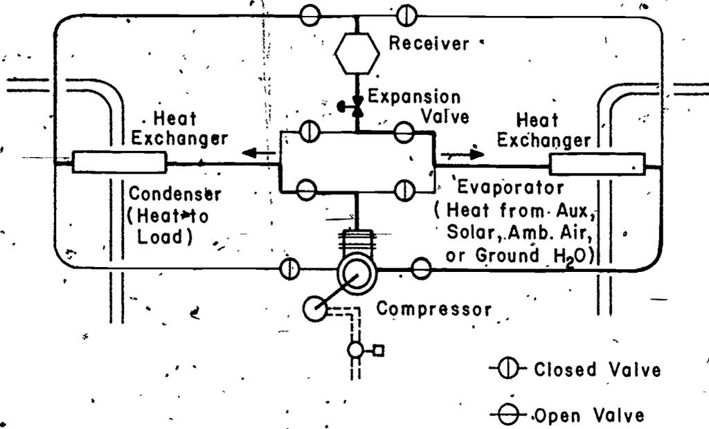
Figure 8-12. Heat Pump in Heating Mode
