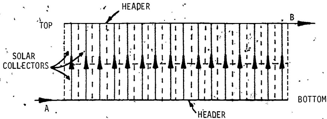
Figure 5-4. Definition Sketch for Fluid Flow Distribution, A Solar Collector Array
