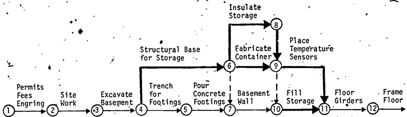
Figure 19-1. Part 1 - Pebble-Bed Storage Fabrication\*
