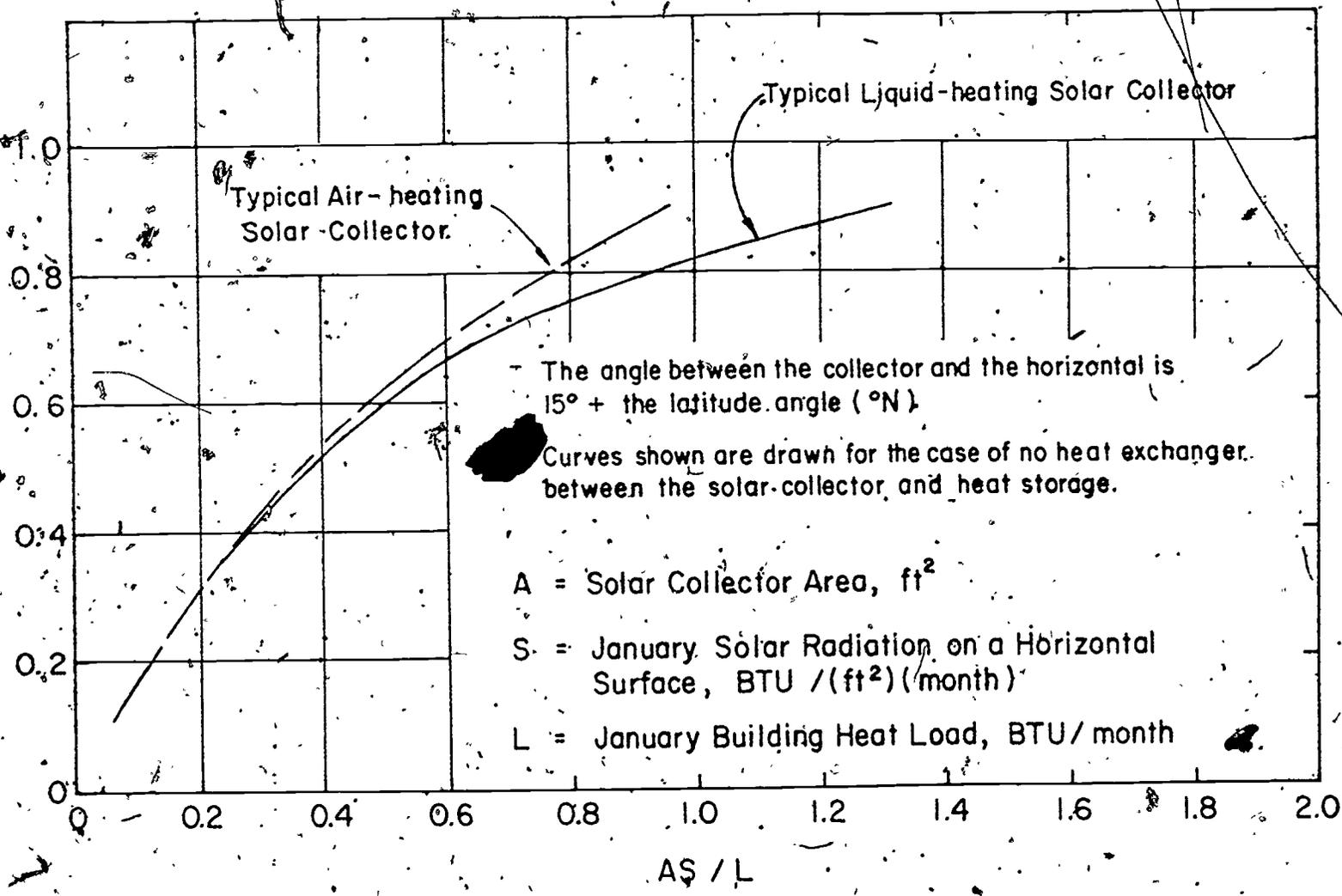
Figure 14-1. Fraction of Annual Heating Load Furnished by a Solar Heating System
