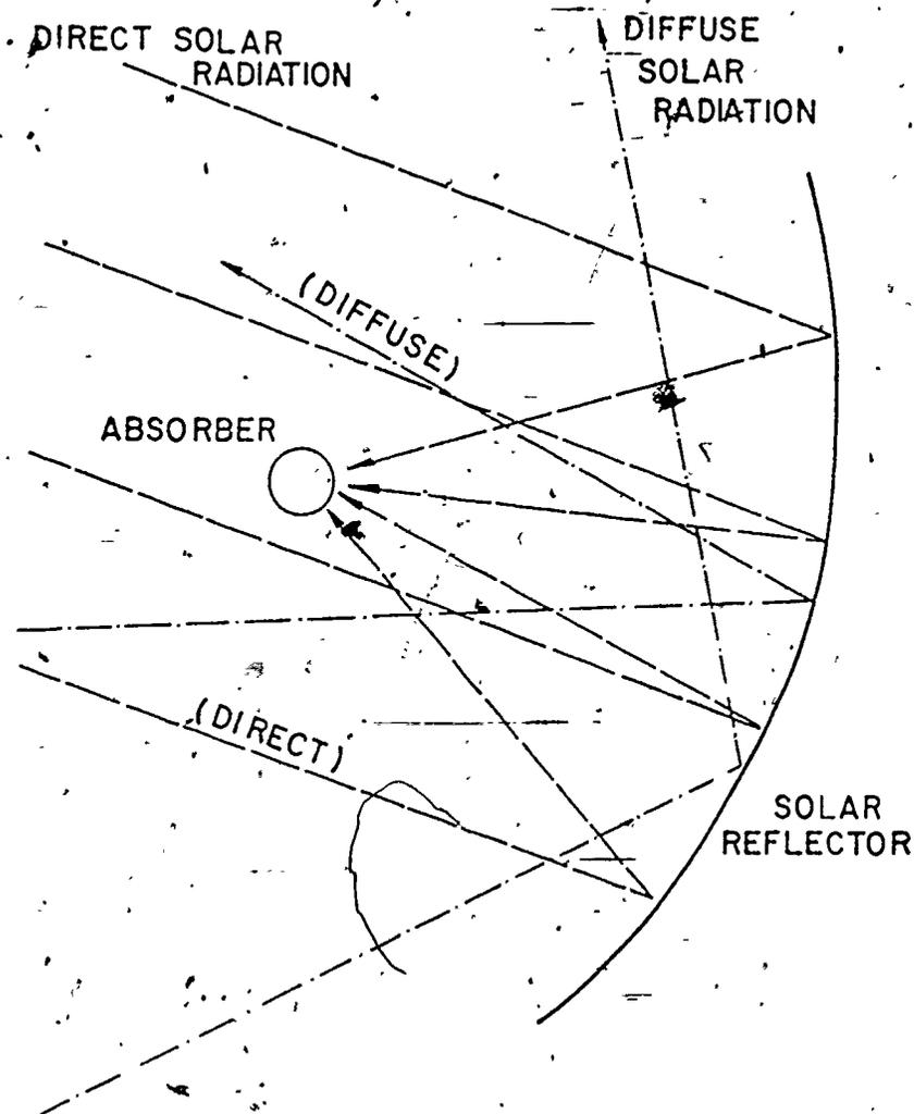
Figure 3-6. - Direct and Diffuse Radiation on a Solar Concentrator
