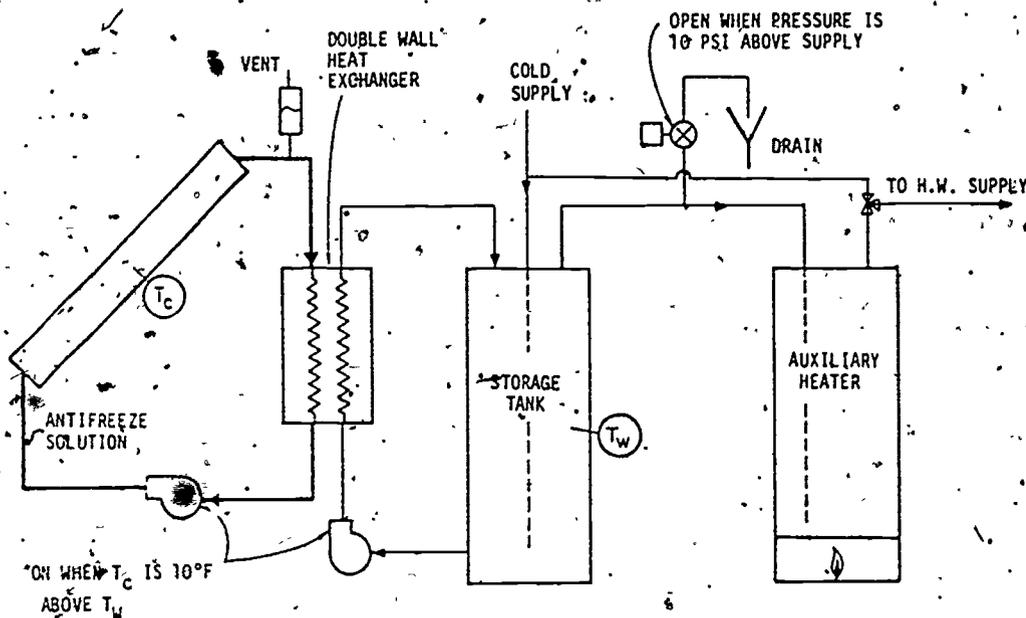
Figure 7-5. Dual-Liquid Solar Hot Water Heater
