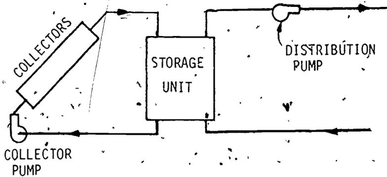
Figure 8-2. Water System Arrangement for Solar Space Heating
