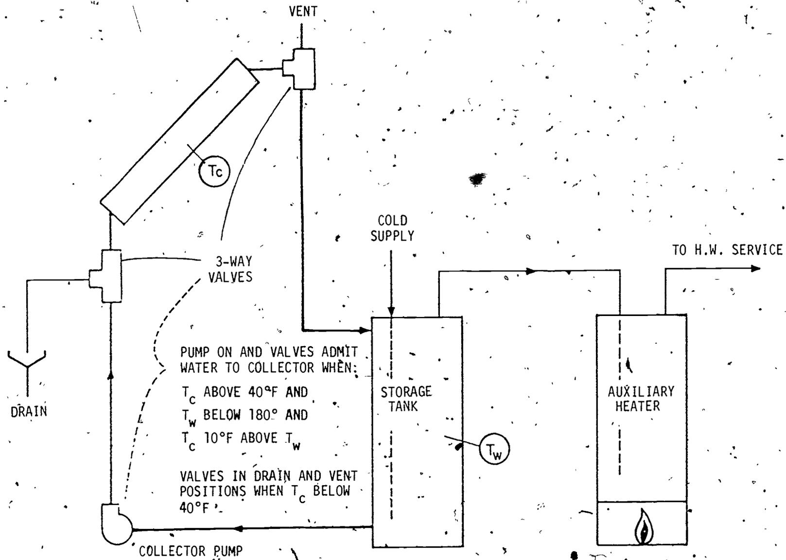
Figure 7-3. Solar Water Heater with Freeze Protection by Automatic Collector Drainage
