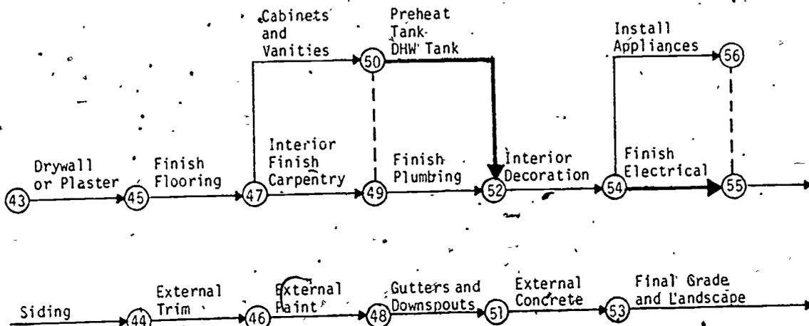
Figure 19-5. Part 5 - Preheat Tank Installation
