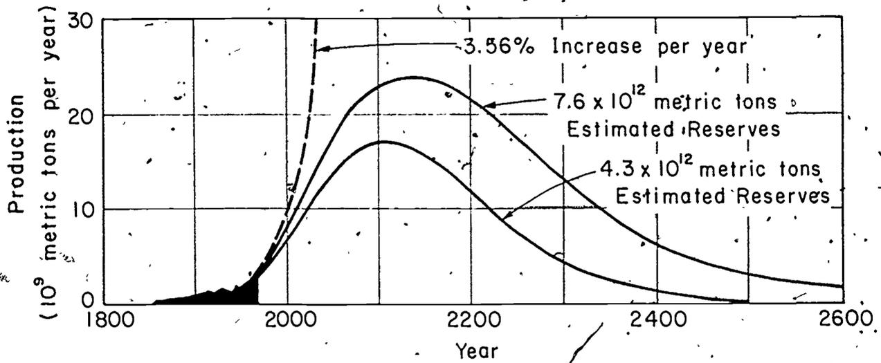
Figure 1.4. Cycle of World Coal Production
