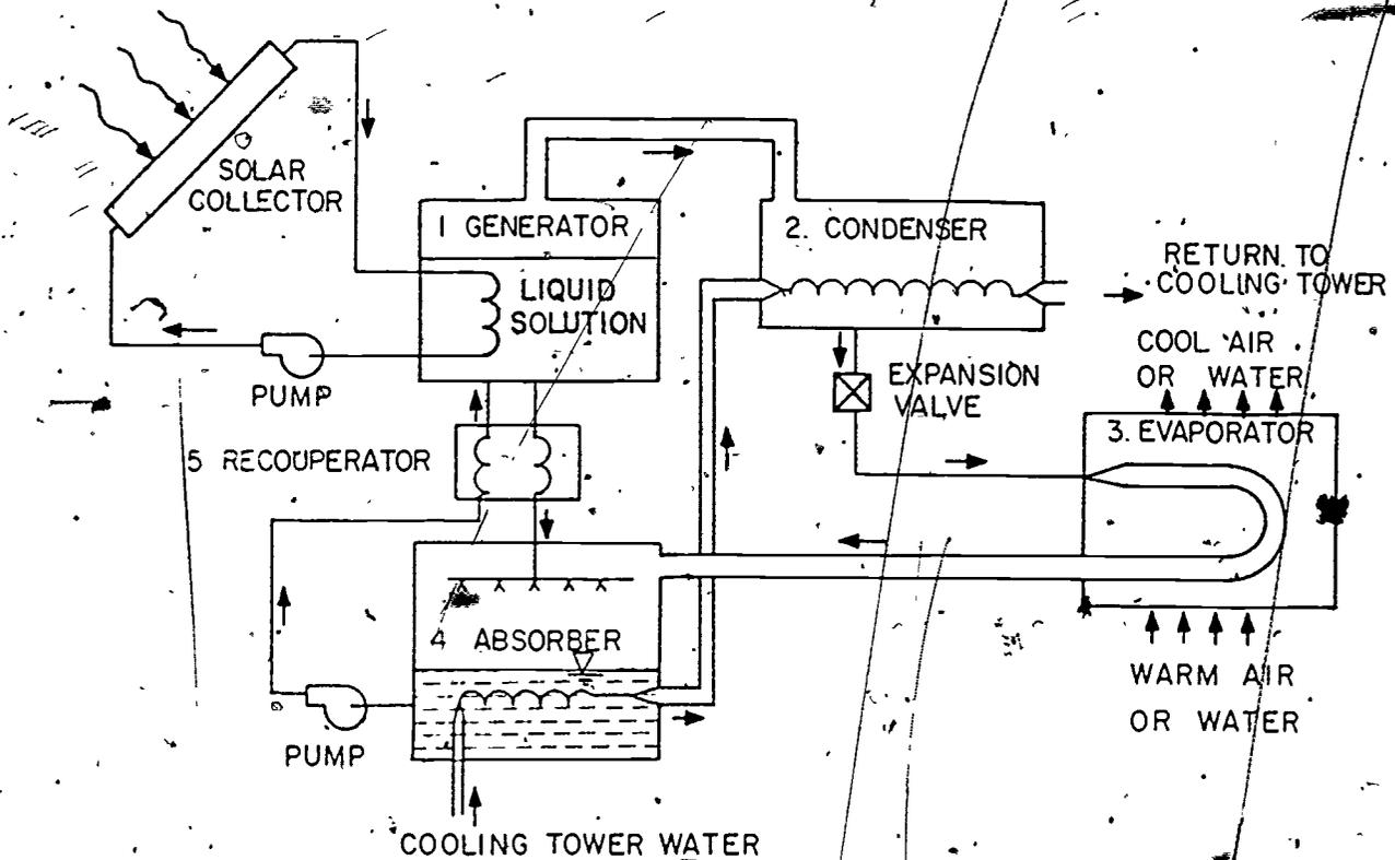
Figure 9-1. Absorption Air Conditioner -- Schematic Drawing
