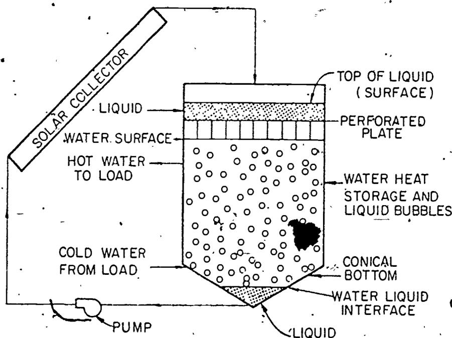
Figure 22-4. Direct Contact Liquid-Liquid Heat Exchanger
