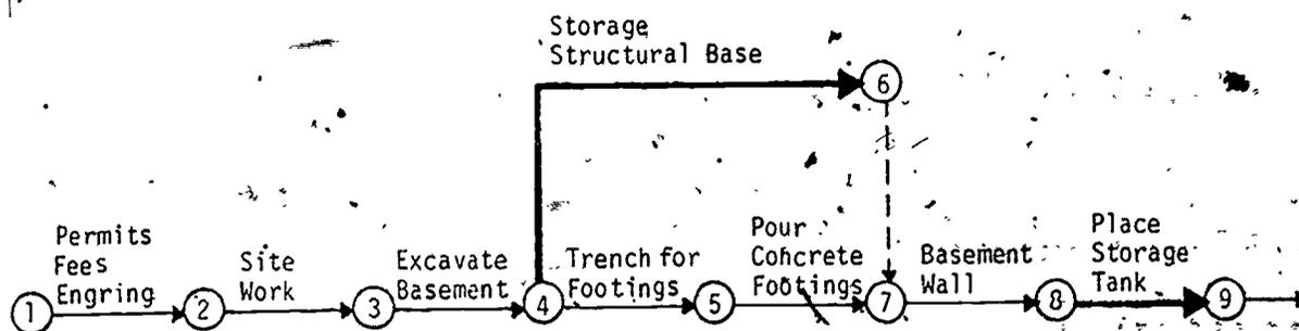
Figure 19-7: Part 1 - Storage Tank Foundation
