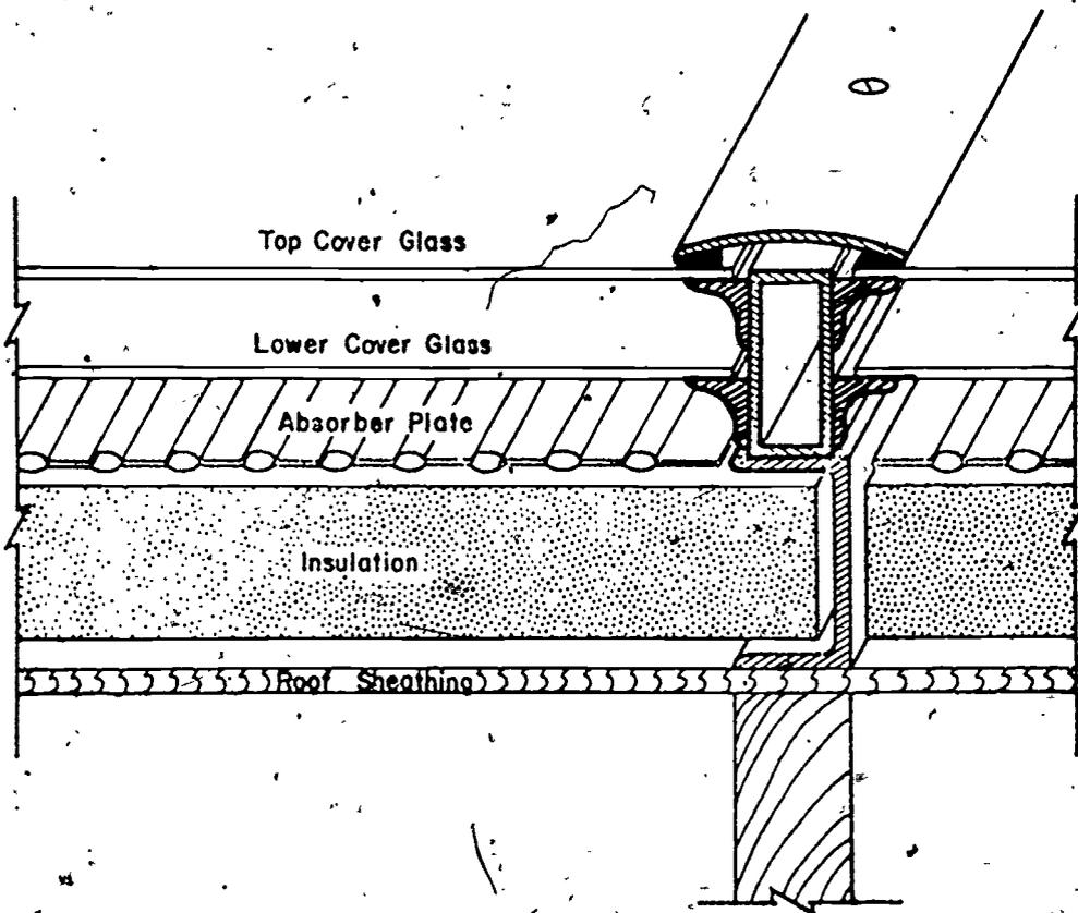
Figure 5-1. Solar Collector Cross-Section
