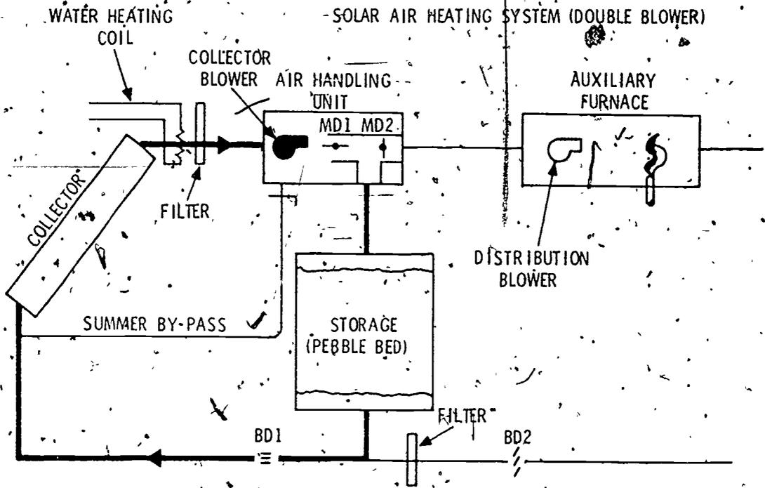
Figure 8-6. Storing Heat from Collectors
