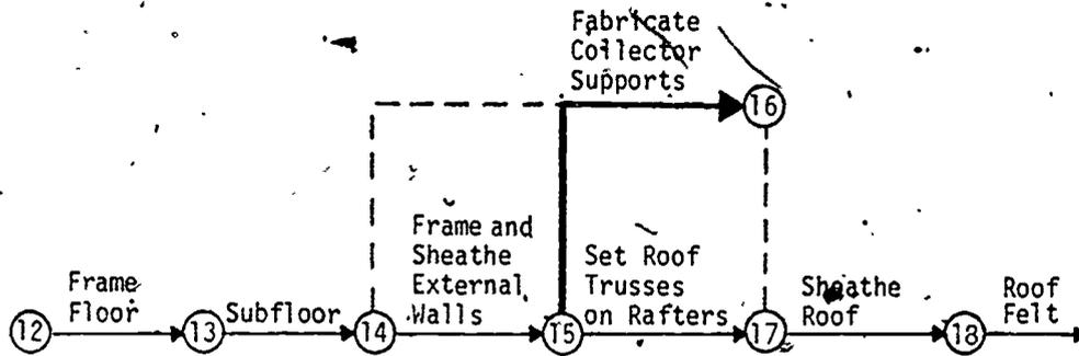
Figure 19-2. Part 2 - Collector Support Construction
