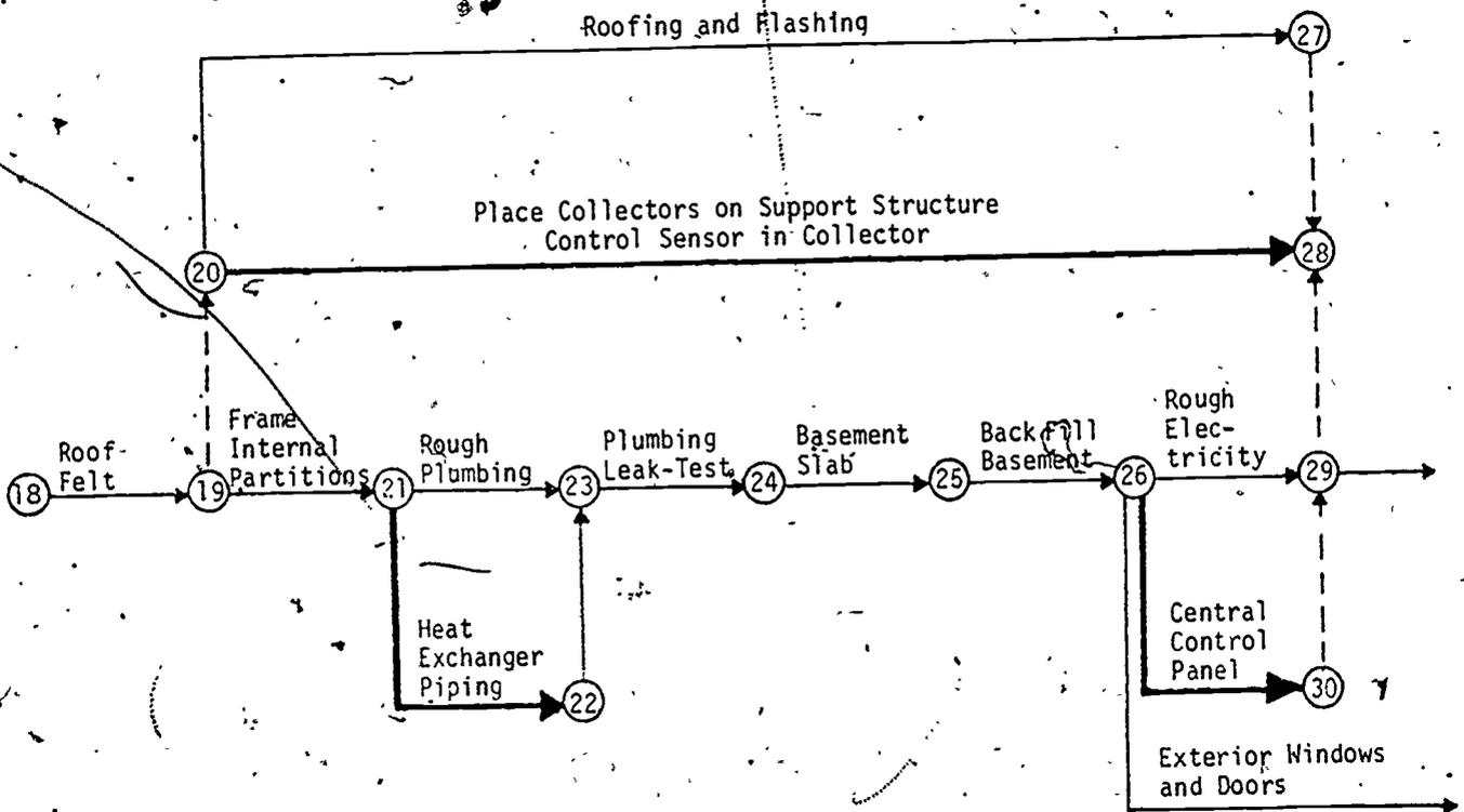
Figure 19-3. Part 3 - Collector, Heat Exchanger, and Control Panel Installation
