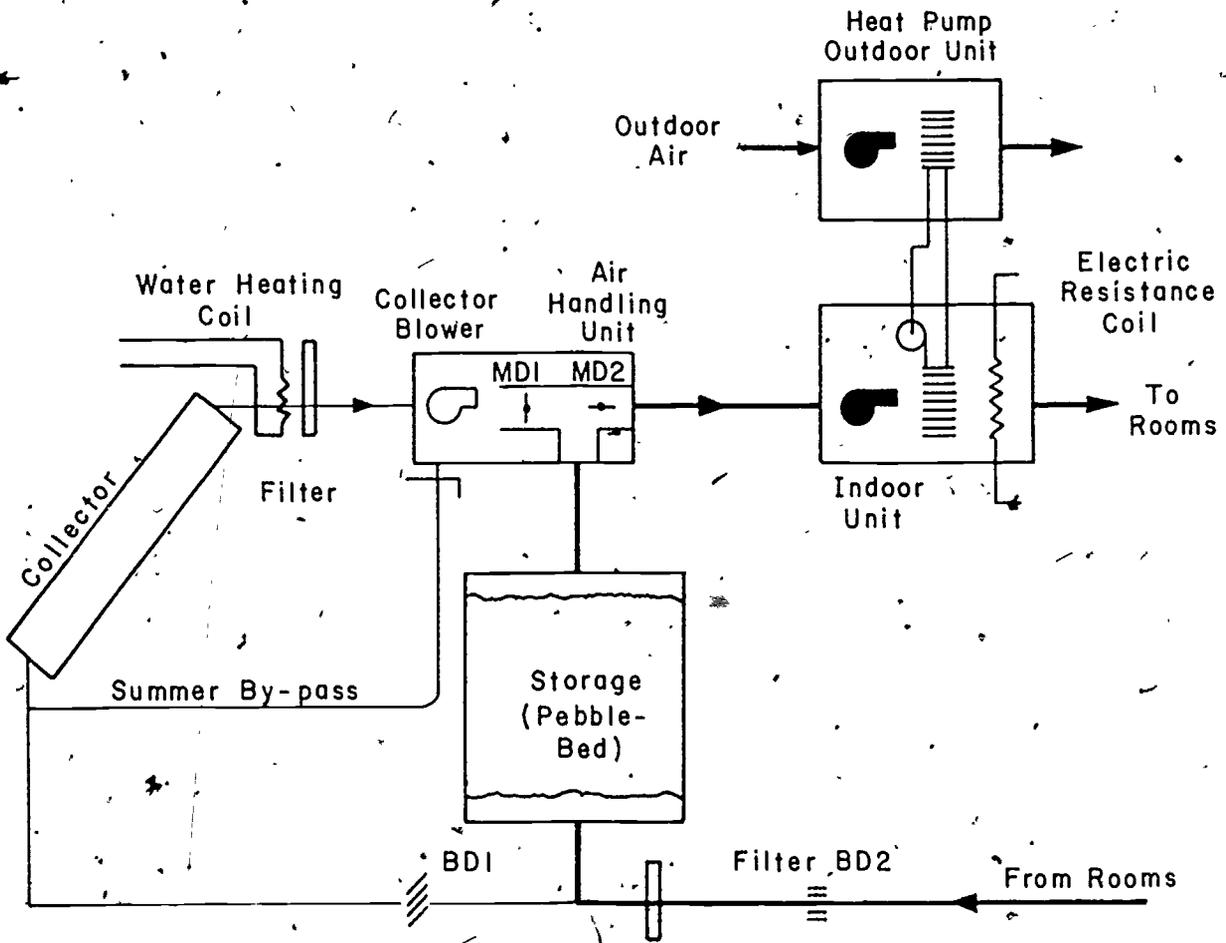
Figure 8-15. Solar Heating System with Air-to-Air Heat Pump Auxiliary (Heating Building from Storage with Heat Pump Supplementary Supply)
