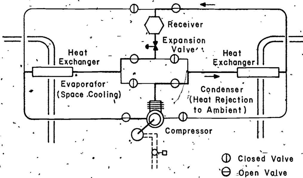
Figure 8-13. Heat Pump in Cooling Mode
