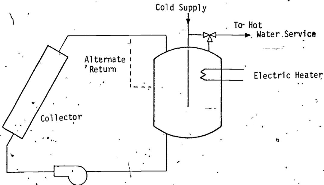
Figure 7-2. Direct Heating, Pump Circulation Type of Solar Water Heater
