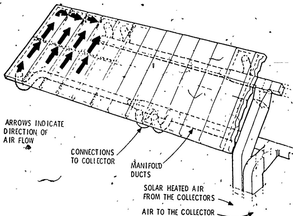
Figure 5-8. Typical Arrangement of Internally Manifolded Collector Modules in an Array
