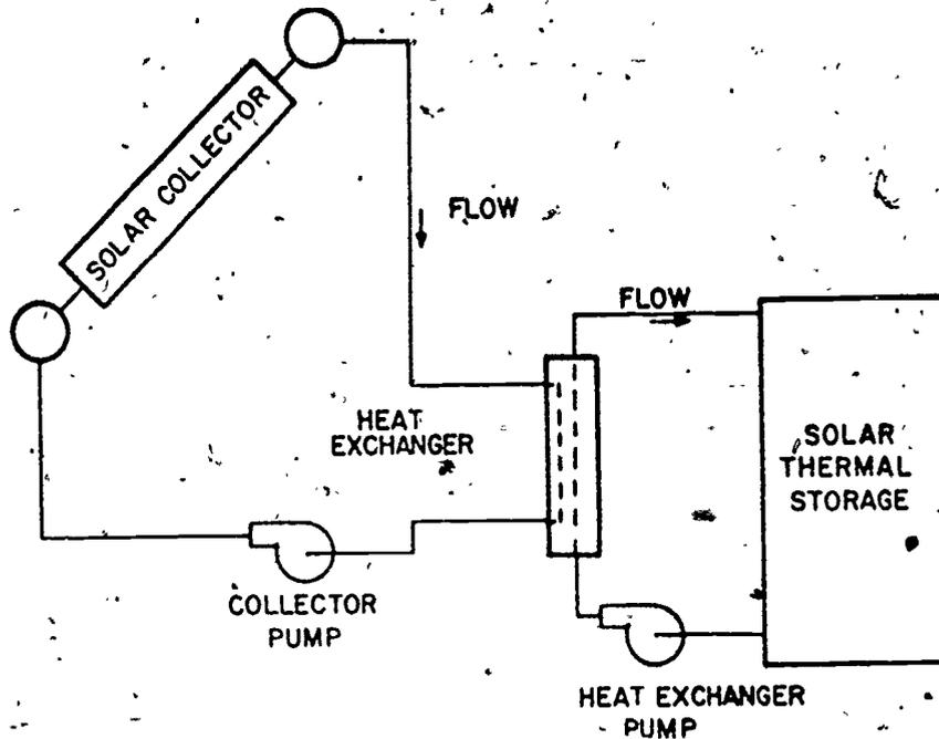
Figure 3-13. Collector Loop with Heat Exchanger
