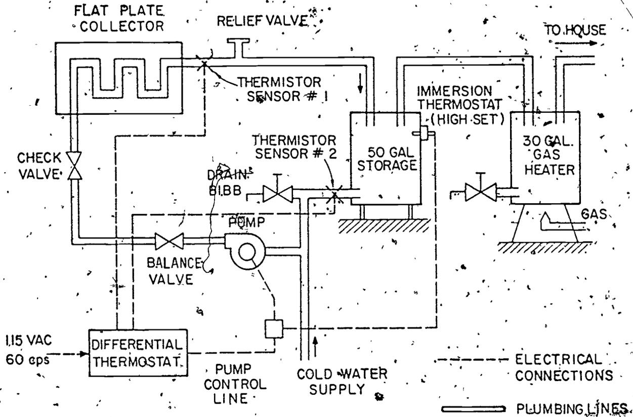
Figure 3-17. Typical Solar Hot Water Control System
