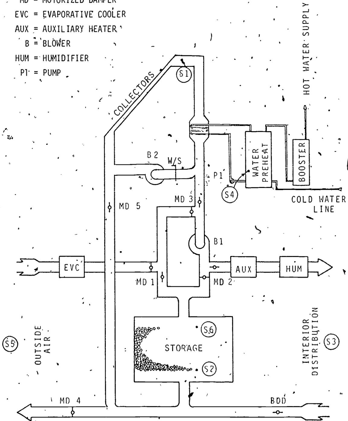
Figure 11-7. Schematic of an Air System (Sensor Locations)
