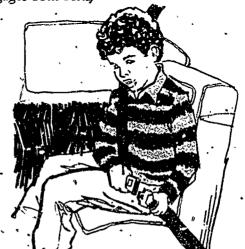
Newer systems have a combination lap and shoulder belt using a single buckle. Both belts are self-adjusting. An inertia reel that locks the belt when the tar makes a sudden stop or during an accident is connected to the shoulder belt.
