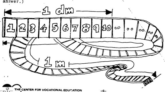
You can get another idea of the size of a centimetre in the picture here. This picture shows a metre, a decimetre, and a centimetre. The symbol <u>cm</u> is used for centimetre. So, if something is 7 centimetres long, you could write this as 7 cm. Make sure you put a space between the numeral (7) and the symbol (cm). No period is placed after any of the metric symbols unless they are at the end of sentences. It is correct to write 7 cm but 7 cm. would not be correct.
