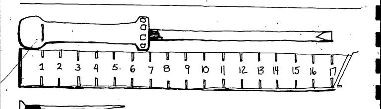
Before you begin the Metric Activities section you are going to have a brief lesson on reading a metric ruler. Look at the picture of the screwdriver next to the metric ruler. One end of the screwdriver is at the end of the ruler near the numeral 1. The other end of the screwdriver is at the 17 mark. This means that the screwdriver is 17 cm long.
