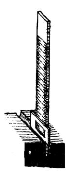
Test Method: Determine past performance, if possible. Test by locating at least one heavy load in the room (e.g. a desk, bookcase, file cabinet, etc.). Observe the floor around the legs from a distance of one foot noting any change in physical condition. If possible, shift the load and observe an indentation in the flooring. Measure this with a depth gauge.
