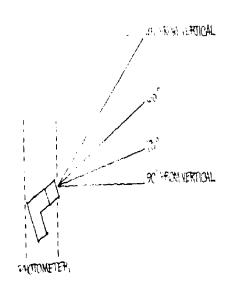
Test Method: Determine past performance, if possible. Use a spectra photometer reading in footlamberts or a (Minolta, Honeywell, etc.) lightmeter whose readings can be converted to footlamberts. Readings are taken with a 1° spot.
