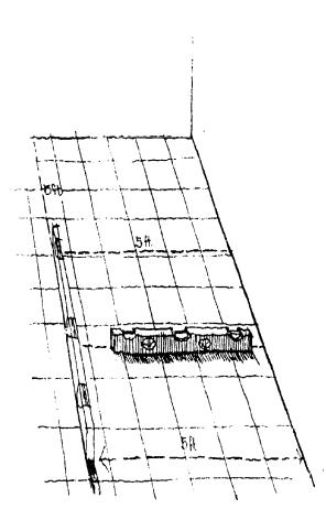
Test Method: Determine past performance, if possible. iest by sweeping the floor clean of all particulate marter which might interfere with the testing procedures. Rolling a spherical object such as a ball bearing to observe deviation from a straight line path, or observing flow or ponding of water during cleaning operations can be used as gross indicators of a general or localized non-level condition which can then be verified by more precise measurement using long levels.
