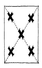
Test Method: Determine past performance, if possible, Test, with a plumbline and a tape graduated to 1/16 inch, by measuring the floor to ceiling height at the one-fifth points of both room diagonals and at the crossing of the diagonals (see diagram). Record each height to 1/16 inch accuracy. Record and photograph.
