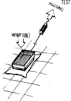
Test Method: Determine past performance, if possible. Test by using a slip meter to determine the coefficient of slip of hard, smooth surfaces (not to be used on carpeting or on heavily-textured surfaces). The slip meter is a weighted cloth bag which is pulled and the force necessary to cause the device to begin moving across a surface is noted on a tension scale. This test need be performed only once for each flooring materia! in use. Record the results for each surface, wet and dry.
