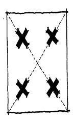
Test Method: The following test is made at the fourth points of both room diagonals. These are used as task locations and the footcandle level is read with and without a user at the task location to compare the possible effects of shadow on the task.
