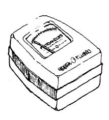
Test Method: [: +ermine past performance, if possible. Use a footcandle meter which reads from 3-8000 footcandles. Multiple readings are take. in each room under luminaires, between luminaires, in the center of the room, at the edge of the room and at the windows. Readings are made under the following conditions - daylight only (between 9 a.m. & 3 p.m.), artificial illumination only (nighttime is best) and a combination of the two. All readings are taken 30 inches above the floor (table height).
