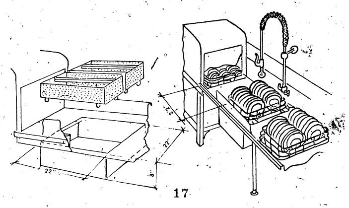
For mechanical pre-rinse, most standard conveyor type dishwashers can be ordered with a built-in pre-rinse. This adds a maximum of two feet to the length of the machine. This is advantageous because the pre-rinse operation is completely automatic, it saves labor and the installation requires less floor space than a pre-rinse sink. The re-circulated pre-rinse is recommended for all conveyor-type dish-machines. The re-circulated pre-wash is recommended in lieu of the fresh water pre-rinse.
