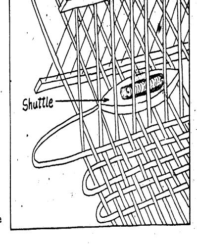
On a loom, crosswise threads from a shuttle were passed over and under the lengthwist threads.
