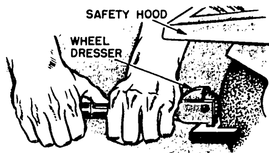
28.63 Figure 5-5.—Using a grinding wheel dresser.
