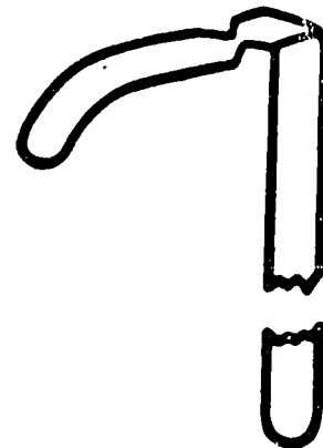
Figure 8-41.— Blown link in plug fuse.
