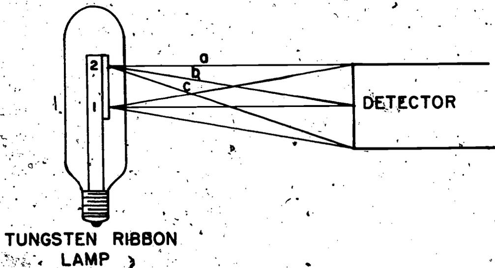
Figure 2.1: Rays from lamp source to detector-receiver.
