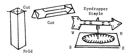
Operation of Equipment: You can use the wooden base with your wind vane almost any place. Just set the glass tubing or medicine dropper over the nail. This type of base can also be mounted on the top of a post by nailing down through the wood. A permanent base can be made from a coat hanger. However, this cannot be moved easily. If you do not wish to leave your weather instruments outside, you need only set up the stand. Then you can quickly set up your wind vane or anemometer to take a reading.
