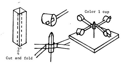
Operation of Equipment: In order to measure the wind speed, count the number of turns in 30 seconds and divide by five. This will give you the wind speed in miles per hour. Each anemometer is a little different. A more accurate way to calibrate the wind speed is to take a ride in a car on a calm day. Stick your anemometer out the car window and count how many times it turns in 30 seconds at, say, 5 miles an hour. Then count the number
