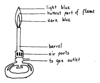
Hoo! burner to gas source. Light match, then turn on gas. Hold match  ${\bf l}$  cm above barrel to ignite. Adjust flame by turning the section of burner where air ports are near base of burner.
