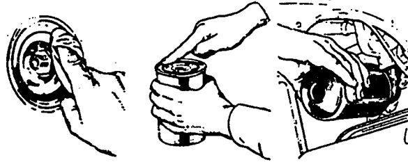
A -- clean base B -- oil seal gasket C -- tighten
