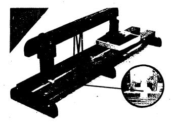
A pushing action. Apparatus being used to break a wood joint while testing the holding power of certain glues.
