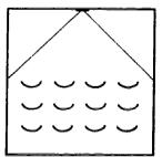
Glass Beaded Screen.—The glass beaded screen gives a comparatively narrow viewing angle, approximately 60 degrees. Within its viewing area, the image is brilliant but outside its viewing area the quality of the image and the amount of light falls off rapidly. A beaded screen is most effective in long, rectangular rooms. If a beaded screen is used in a square room, it is likely that the seats on the front cor-
