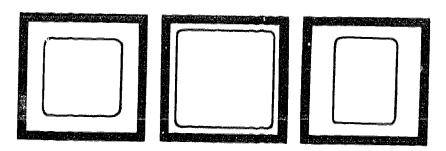
2" x 2" cardboard mounts are 35mm, 127 film, and the Instamatic (126). Each of these produces a slightly different size projectable film within the 2" x 2" mount (See illustration).
