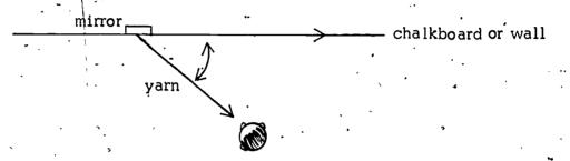
The projector must be placed so that the angle formed by the chalkboard and the light beam equals the angle formed by the chalkboard and the yarn.
