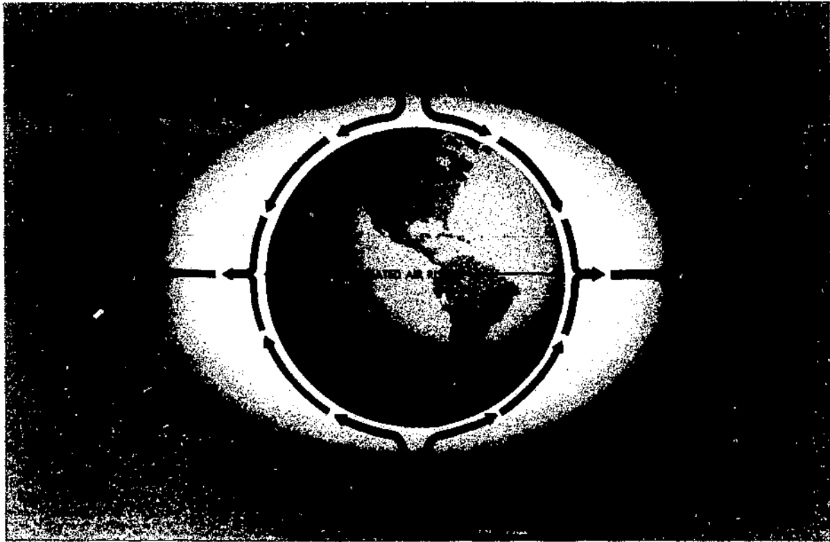
FIGURE 19. Circulation as it would be on a nonrotating globe. Intense heating at the Equator lowers the density. More dense air flows from the poles toward the Equator forcing the less dense air aloft where it flows toward the poles. The circulation would be two giant hemispherical convective currents.
