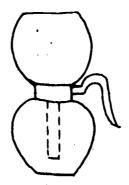
The vacuum coffee maker has a glass or metal upper bowl and a glass or metal lower bowl. The neck of the upper bowl fits through the opening of the lower bowl to form a tight seal. Vacuum coffee makers range in size from a single burner unit to a terraced unit with eight burners and decanters. The decanters hold 10-12 cups, or 1/2 gallon of coffee.
