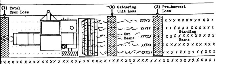
et in from ends of field and where crop is typical of entire it 15 feet. Place rectangular frame across swath harvested ill beans in frame and enter this count in loss data table ber by 40 and enter the loss in bushels per acre in columnid, keep right on harvesting. If loss is greater, then proceed iss.
