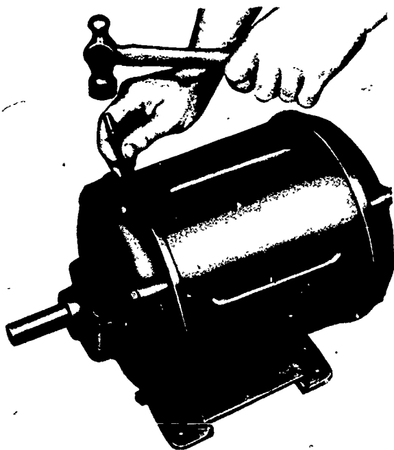
73.223 Figure 8-19.—Marking a motor frame and end bell.
