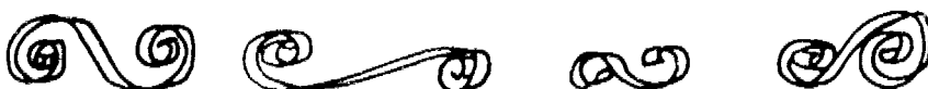
made by rolling opposite ends in opposite directions differing amounts (S shapes)
